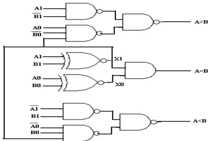
Figure 2. Logic Diagram of 2-Bit Magnitude Comparator
