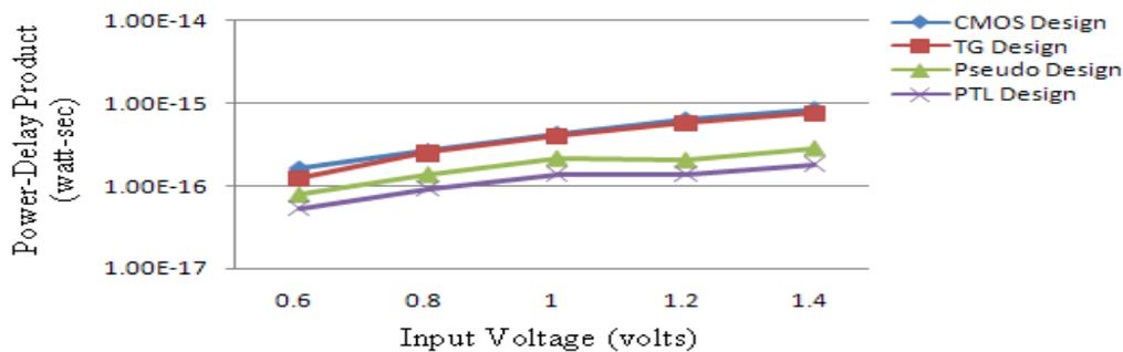
Figure 17. Power-Delay Product vs Input Voltage
