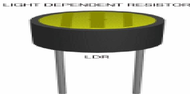
Figure 4: Light Dependent Resistor
