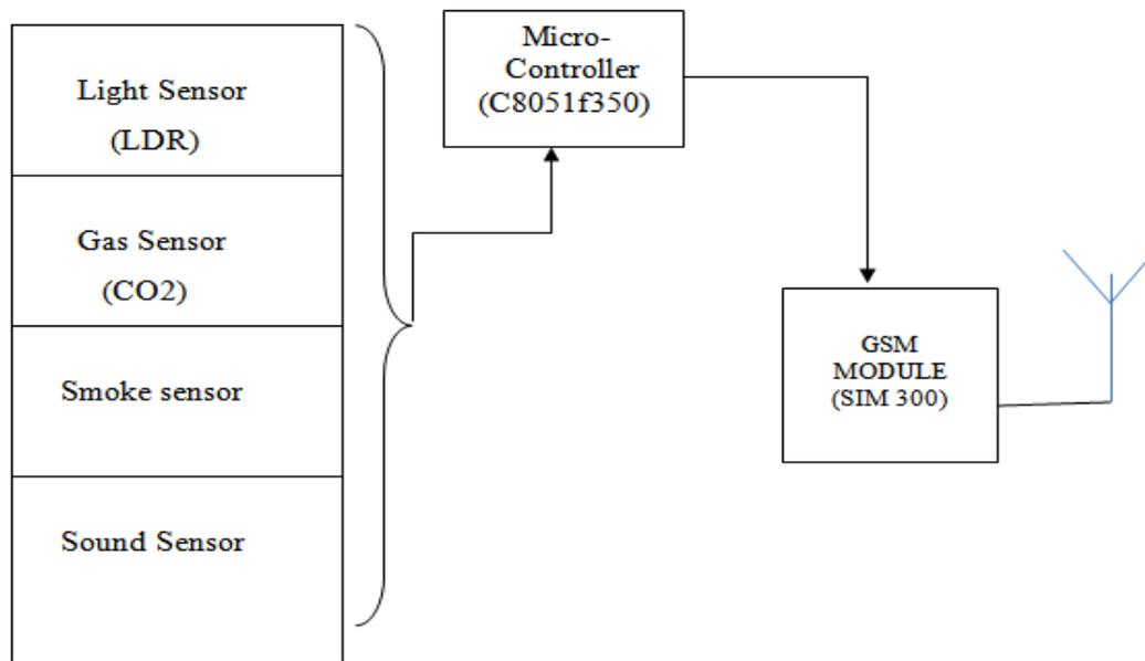
Figure 2: Block Diagram Transmission Side
