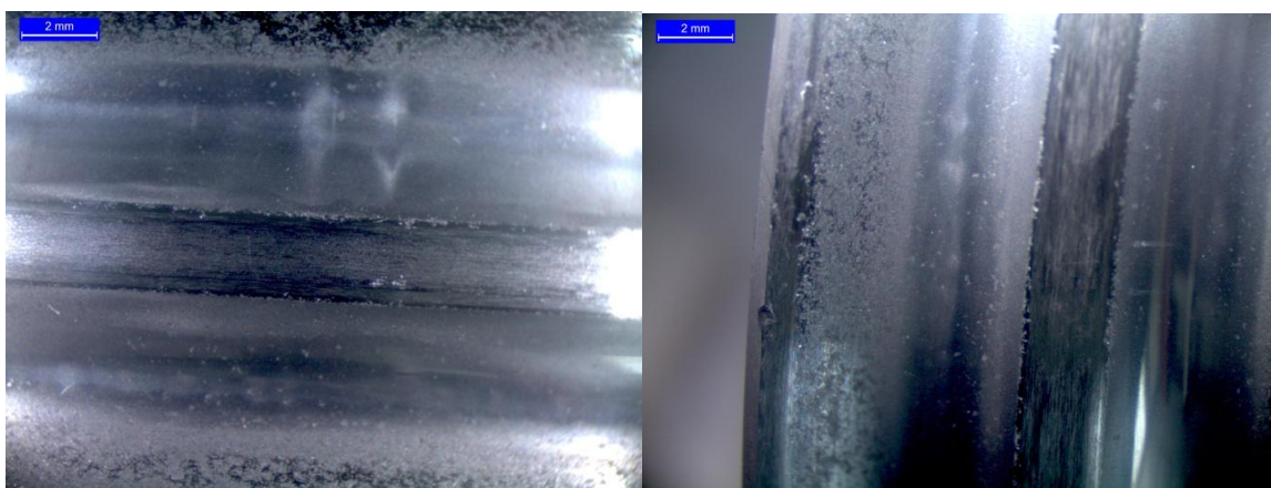
Figures 6a & 6b: Deformations on the inner raceway on the bearing raceways of the 3 rd case.
