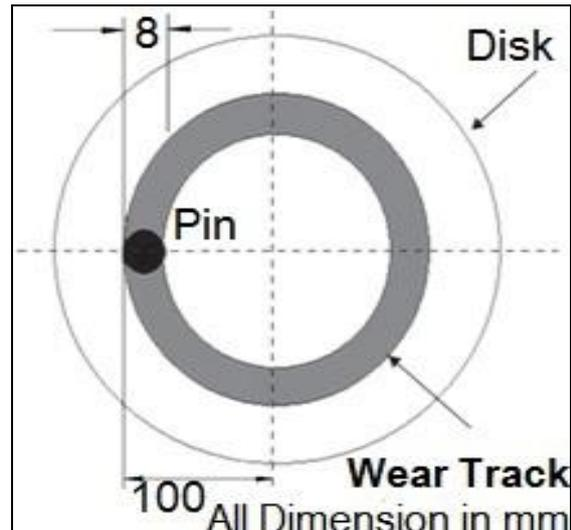
Fig.2. Schematic diagram of Wear Test
