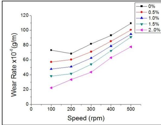
**Fig.8.**Wear Rate Vs Speed for Different Wt. % Reinforcements for constant Load 30N and Constant Time of 300 Sec
