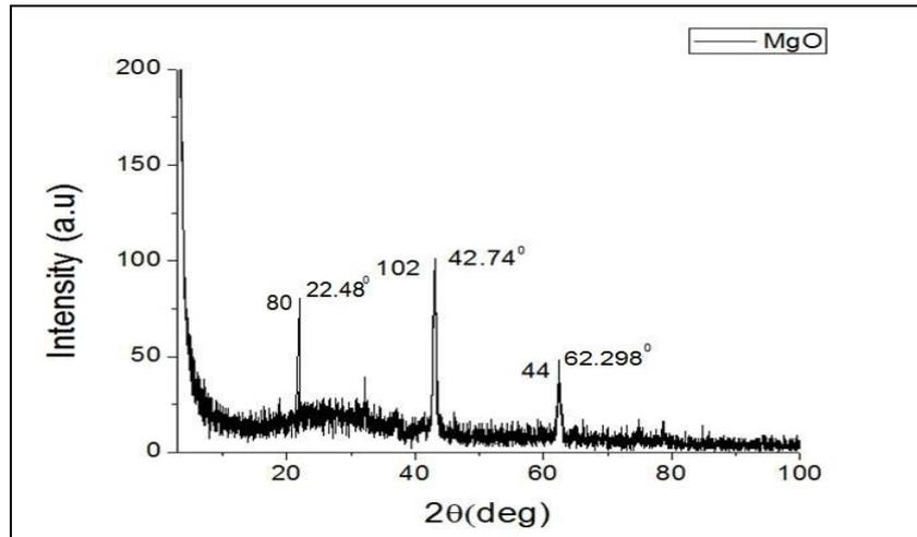
**Fig.3.** XRD pattern of MgO Nano powder fabricated at  $850 \pm 5^\circ\text{C}$
