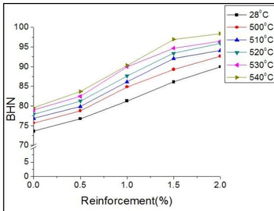
Fig.4. BHN Vs Wt. % Reinforcements at varying temperatures
