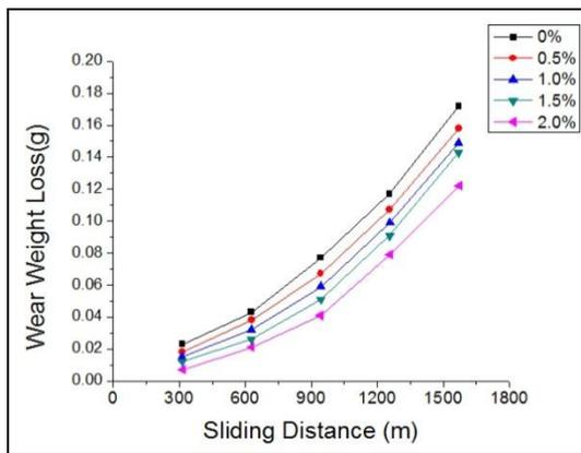
Fig.6. Wear Weight Loss Vs Sliding Distance for Different Wt. % Reinforcements for constant Load 30N and constant Time of 300 Sec.
