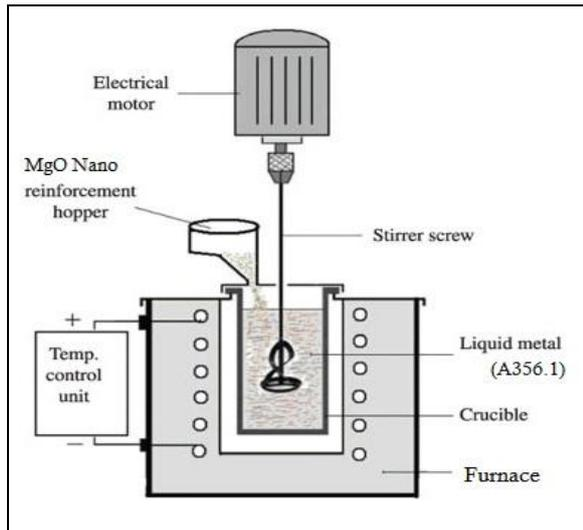
Fig.1. Schematic diagram of Stir Casting technique
