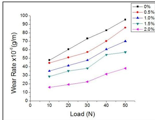
Fig.7. Wear Rate Vs Load for Different Wt. % Reinforcements for constant Speed 300rpm and constant Time of 300 Sec
