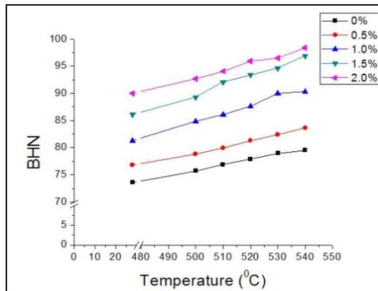
Fig.5. BHN Vs Temperature for Different Wt. % Reinforcements.
