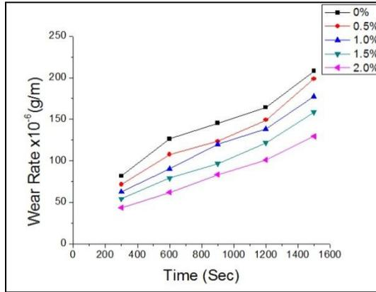
**Fig.9.**Wear Rate Vs Time for Different Wt. % Reinforcements for constant Load 30N and Constant Speed of 300rpm
