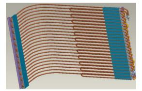
Fig- 4: Typical Plate Finned-Tube Heat Exchanger
