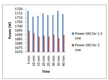
Comparison of Power for 1.5 row and 2 row condenser with respect to time.
