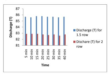
Comparison of Discharge (T°) with 1.5 Row and 2.0 Row Fin Tube Condenser heat Exchanger
