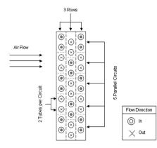
Fig-6: General Heat Exchanger Dimensions[23]
