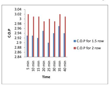
Comparison of C.O.P with 1.5 Row and 2.0 Row Fin Tube Condenser heat Exchanger.
