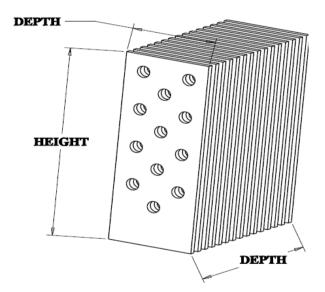
Fig-7: Layout of Heat Exchanger Geometry Parameters[23]
