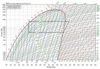
Fig-9: P-H diagram of FIN tube heat condenser with 2.0 row coil on the cooling of 1.5TR split air conditioner.
