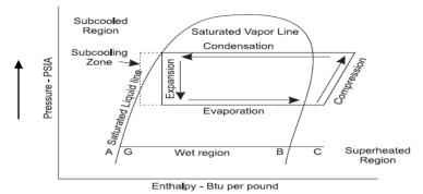
Fig-3: Schematic representation of the refrigeration cycle including pressure change.
