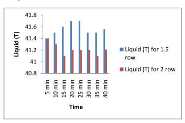
Comparison of liquid temperature with 1.5 Row and 2.0 Row Fin Tube Condenser heat exchanger
