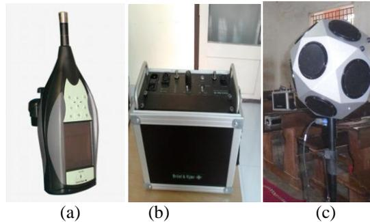
(a) Brüel and kjaer (BK 2250) sound level meter used for measuring Reverberation time. (b) 2734-B power amplifier. (c) 4292-L Omni Power sound source.
