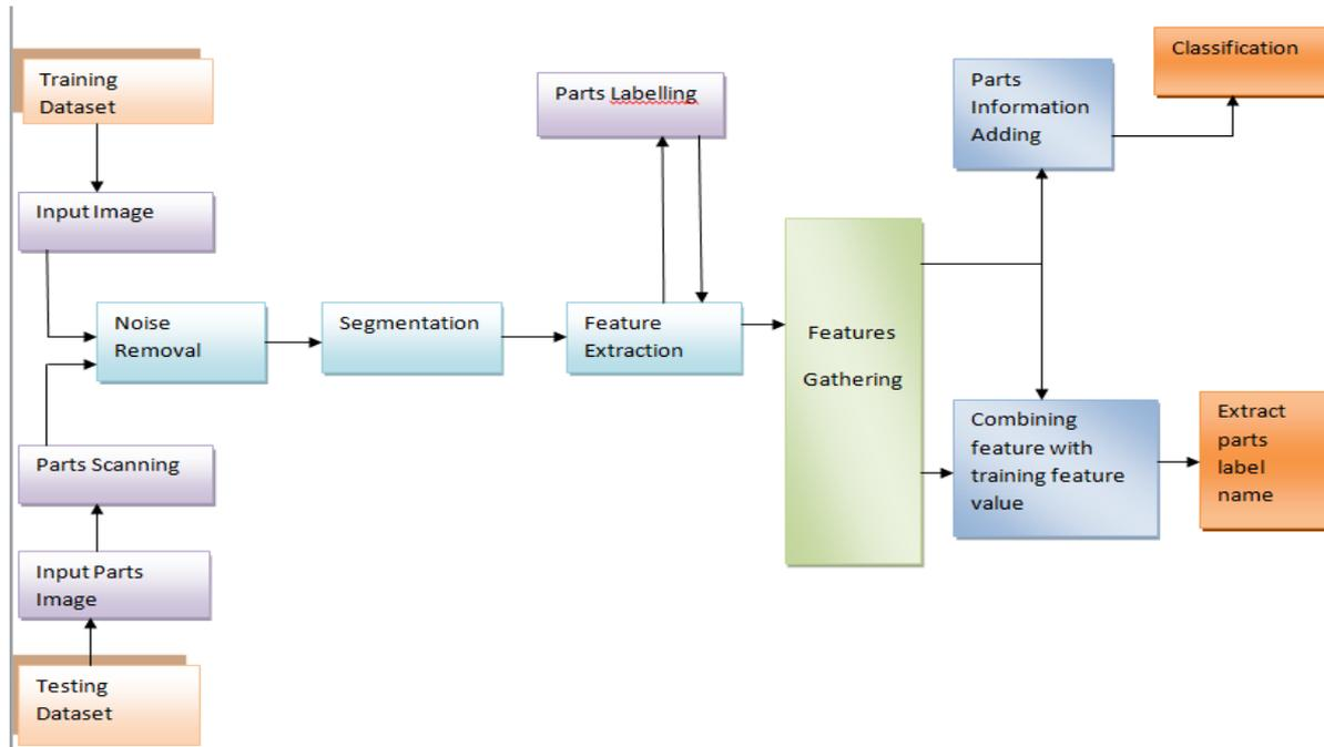
Fig.1 Architecture diagram of the proposed rotation invariant part based model
