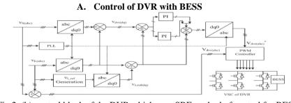
Fig.2. (b) control block of the DVR which uses SRF method of control for BESS
