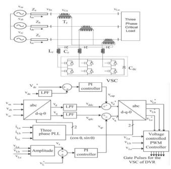
Fig.3. (a) Schematic diagram of a capacitor supported DVR connected system. (b) Control block of the DVR which uses SRF method of control for capacitor connected DVR
