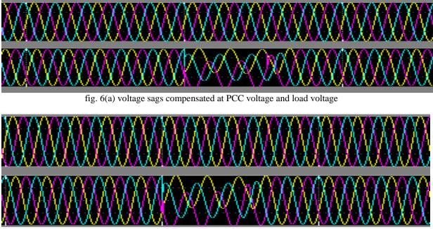
fig. 6(b) voltage swells compensated at PCC voltage and load voltage
