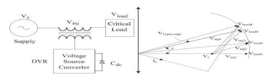
Fig. 1(a): schematic representation of DVR connected system. (b) Phasor diagram of different voltage injection schemes of DVR.
