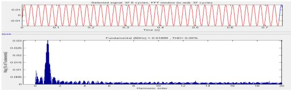
Fig 7(c).input signal and its THD analysis for capacitor supported DVR connected system
