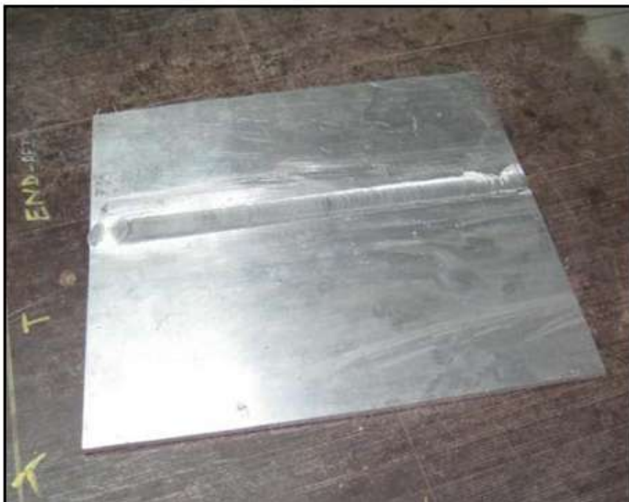
Figure 3.16: FSW of aluminum joint.
