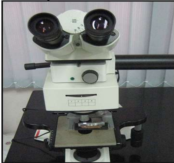
Figure 3.11: Metallographic testing of FSW joints.
