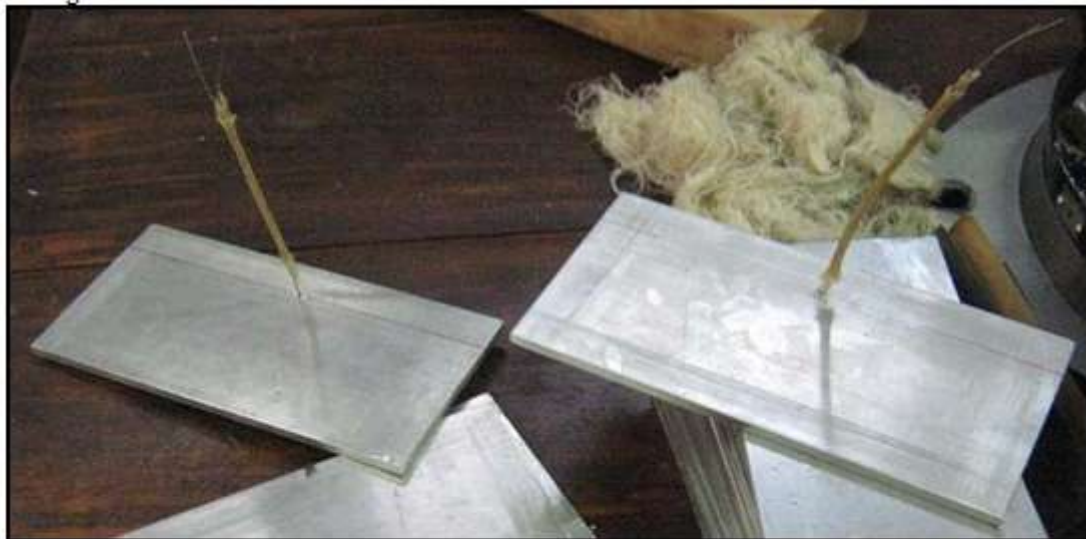
Figure 3.4: Aluminum Plates with Thermocouples.
