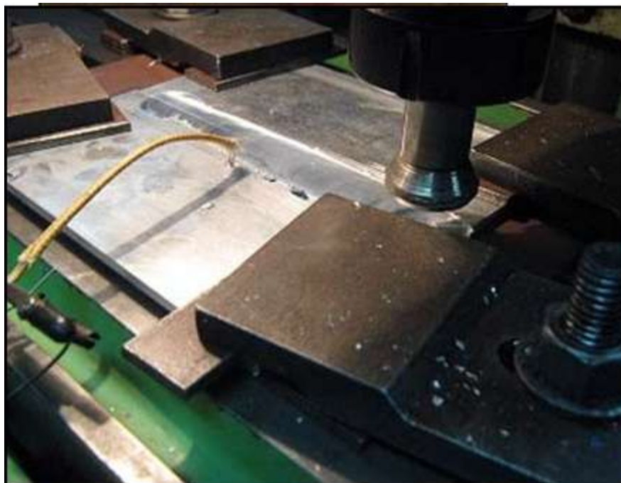
Figure 3.14: FSW of aluminum plate in progress.
