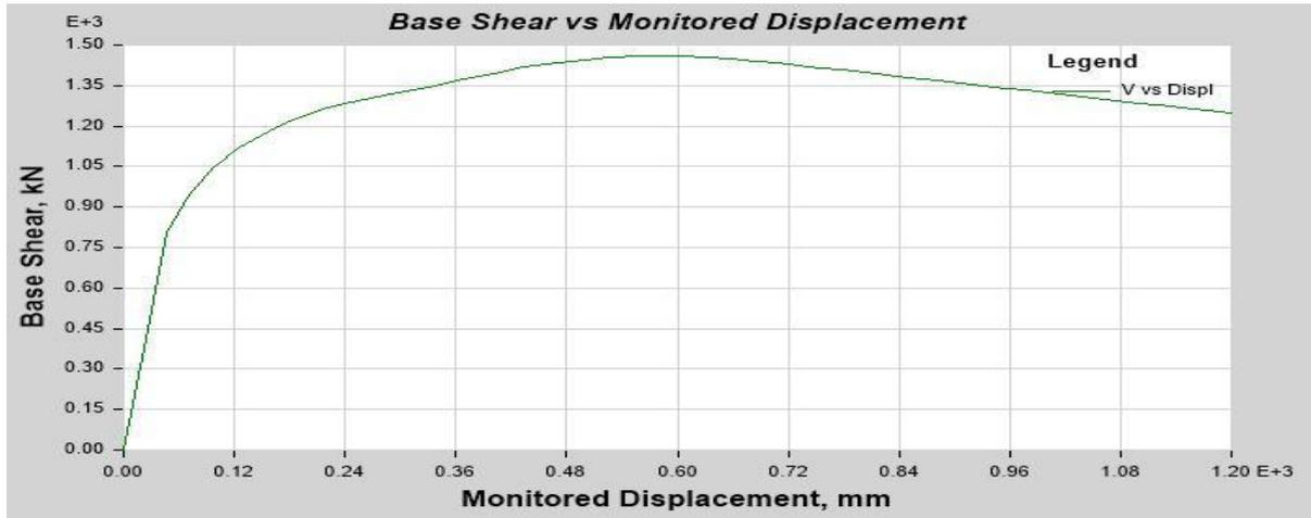
Fig 3.2 Push-Over curve of the model 3 bare frame G+9 building
