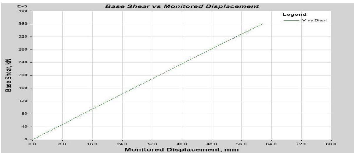
Fig 3.6 Push-Over curve of the Ferro cement infilled frame G+3 building model 5
