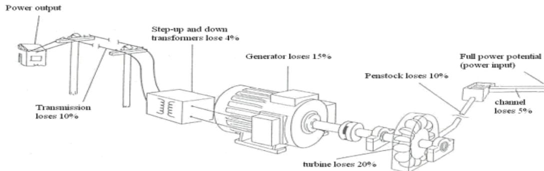
Figure 4: Typical system efficiency of small-hydro power generation [15]
