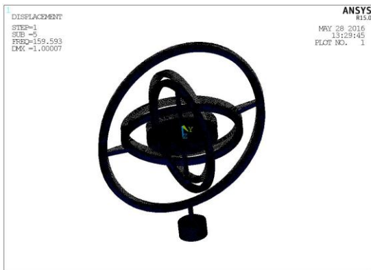
e. 5 th Mode ( f_{n5}=159.593\text{Hz} )
