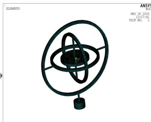
Fig.3: Meshed Model of Gyroscope with Tet Elements
