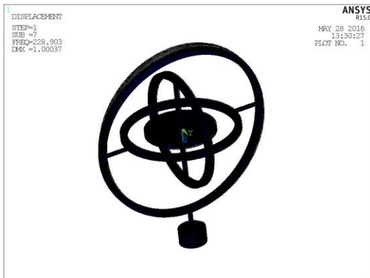
g. 7 th Mode ( f_{n7}=228.9\text{Hz} )
