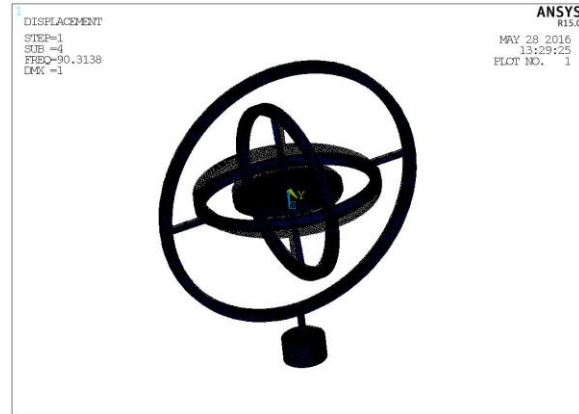
d. 4 th Mode ( f_{n4}=90.3138\text{Hz} )
