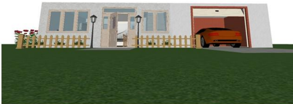
Figure 2: South facing glazed windows for passive solar heating for winter.
