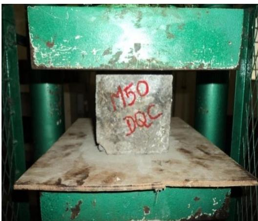
Fig.4 Specimen for Compressive Strength of Cubes
