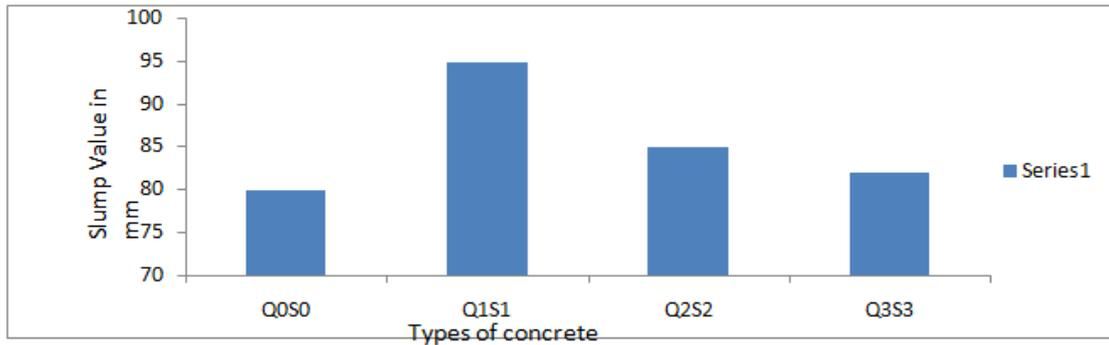
Fig.1 Comparison of Slump Cone Test values
