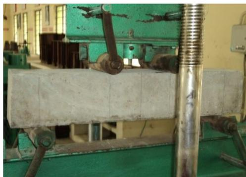
Fig.13 Specimen for Flexural Strength of Beam
