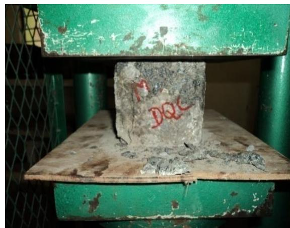
Fig.5 Failure of compressive cube
