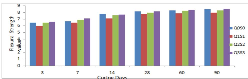
Fig.15 Development of Flexural Strength of Beams
