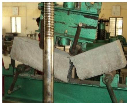
Fig.14 Failure of Beam
