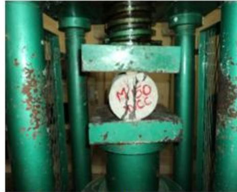
**Fig.10 Specimen for split tensile strength of cylinder    Fig.11 Failure of split tensile Cylinder**
