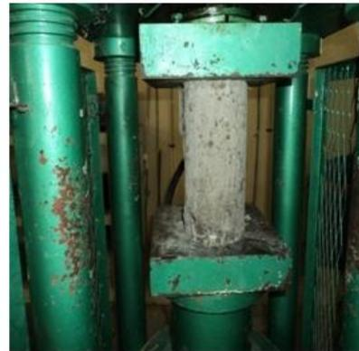
**Fig.8** Failure of Compressive Cylinder
