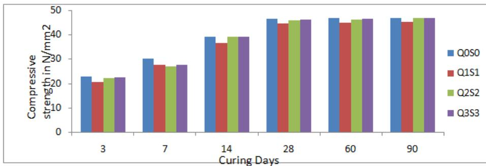
**Fig.9** Development of Compressive Strength of Cylinder
