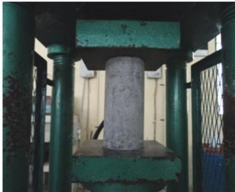
**Fig.7** Specimen for compressive strength of cylinder
