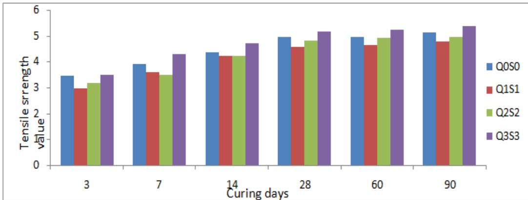
**Fig.12 Development of Split Tensile Strength of Cylinders**
