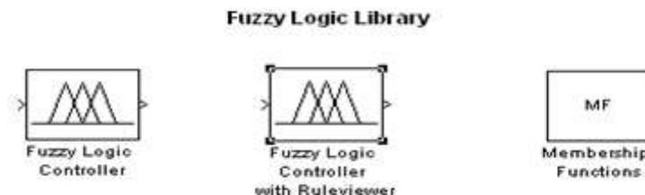
In (Figure 6) this simulink block use for evaluation of FIS and this block shows us how our rules attach with our inputs and output and after defuzzification gives us a single value output and by moving the both inputs we find a change output similarly each point of input we can find output value.
