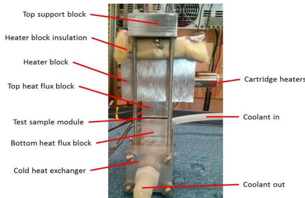
**Fig.2:** Photograph of Test Stand (without Side Insulation)
