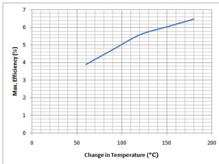
**Fig. 7:** Max. Efficiency Variation with Change in Temperature for Tin Selenid
