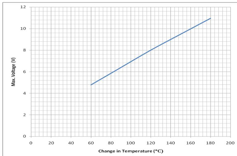
**Fig. 5:** Max. Voltage Variation with Change in Temperature for Tin Selenid Module
