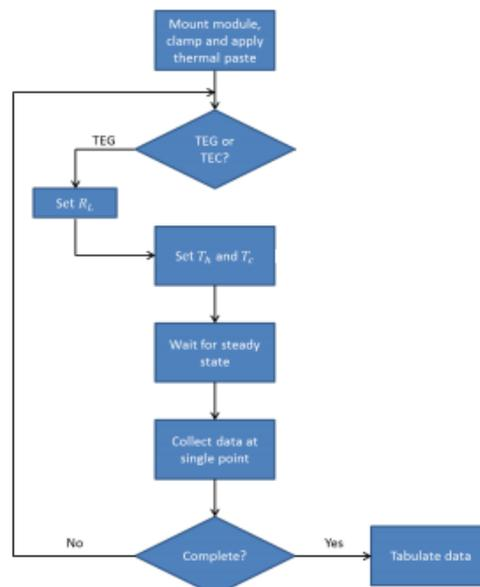
**Fig.3:** Process Flowchart of Experimental Performance Evaluation
