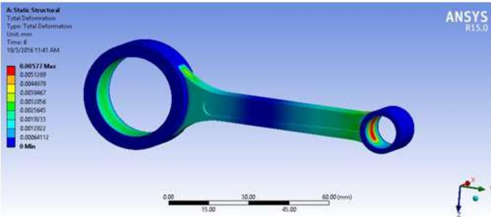
**Fig.17. Total deformation in ASTM A 216 GR WCB connecting rod**
