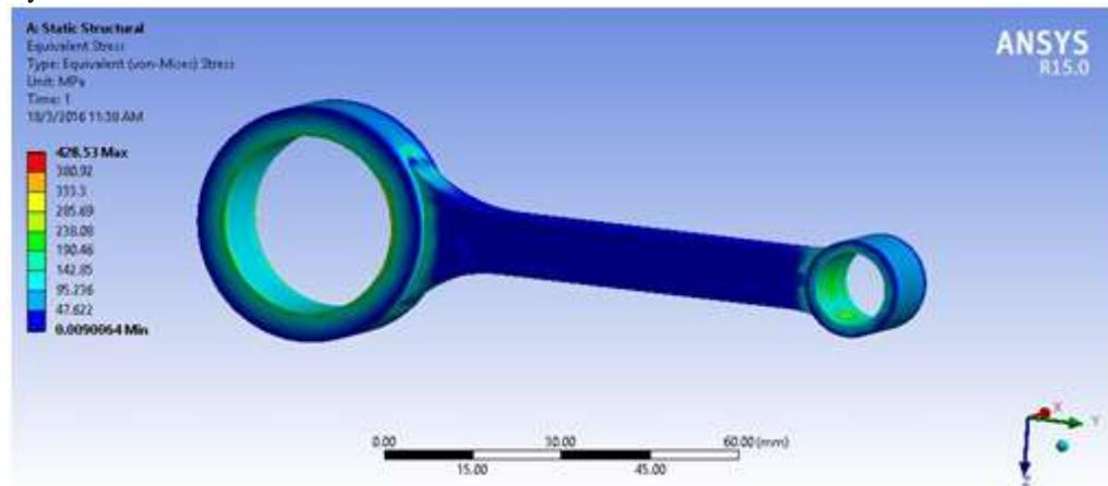
**Fig.15. Equivalent stress in ASTM A 216 GR WCB connecting rod**
