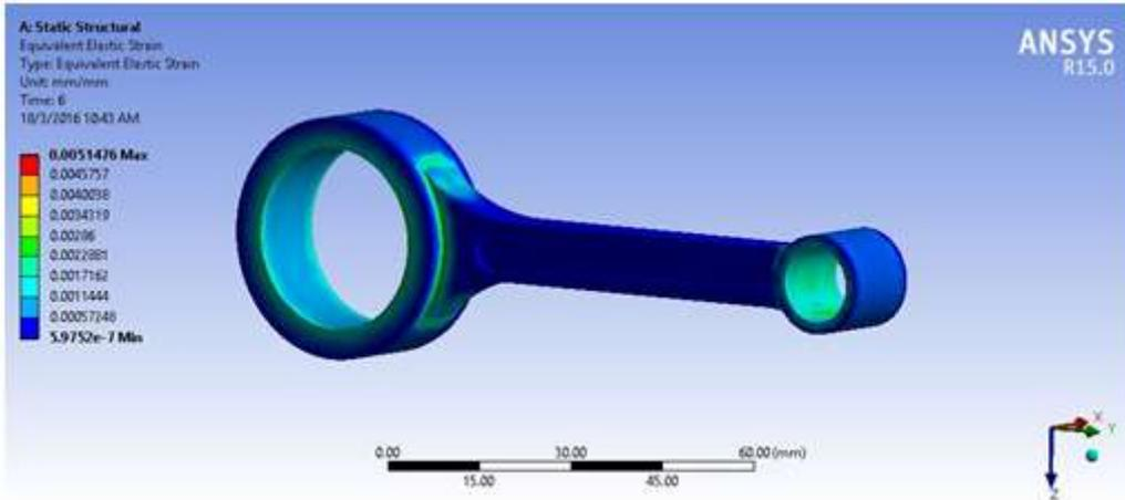
**Fig.13. Equivalent elastic strain in Titanium 6 AL 4V connecting rod**
