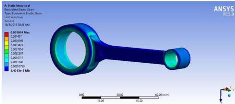
Fig.10. Equivalent Strain in Grey Cast Iron connecting rod
