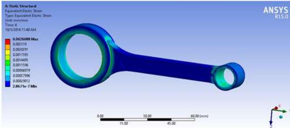
**Fig.16. Equivalent strain in ASTM A 216 GR WCB connecting rod**
