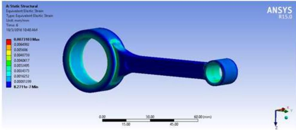
**Fig.7. Equivalent Strain in Aluminum Alloy 6061 connecting rod**
