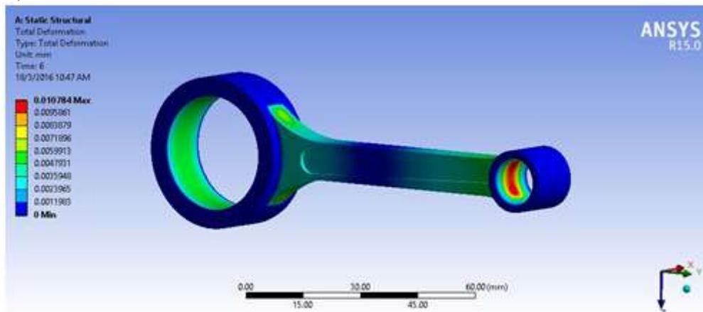
Fig.11.Total Deformation in Grey Cast Iron connecting rod
