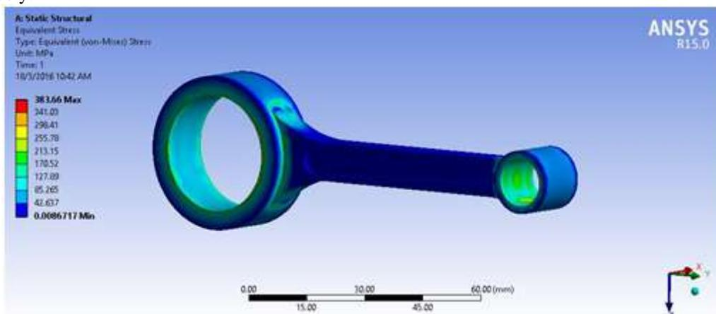
**Fig.12. Equivalent stress in Titanium 6 AL 4V connecting rod**
