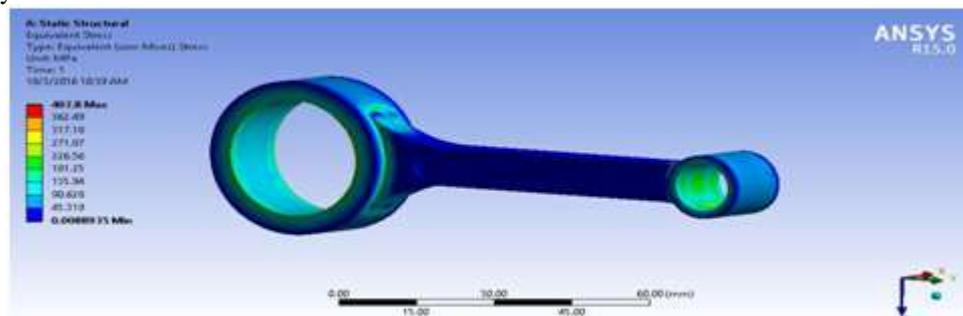
**Fig.6. Equivalent Stress in Aluminum Alloy 6061 connecting rod**
