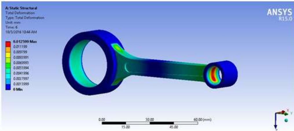
**Fig.14. Total deformation in Titanium 6 AL 4V connecting rod**
