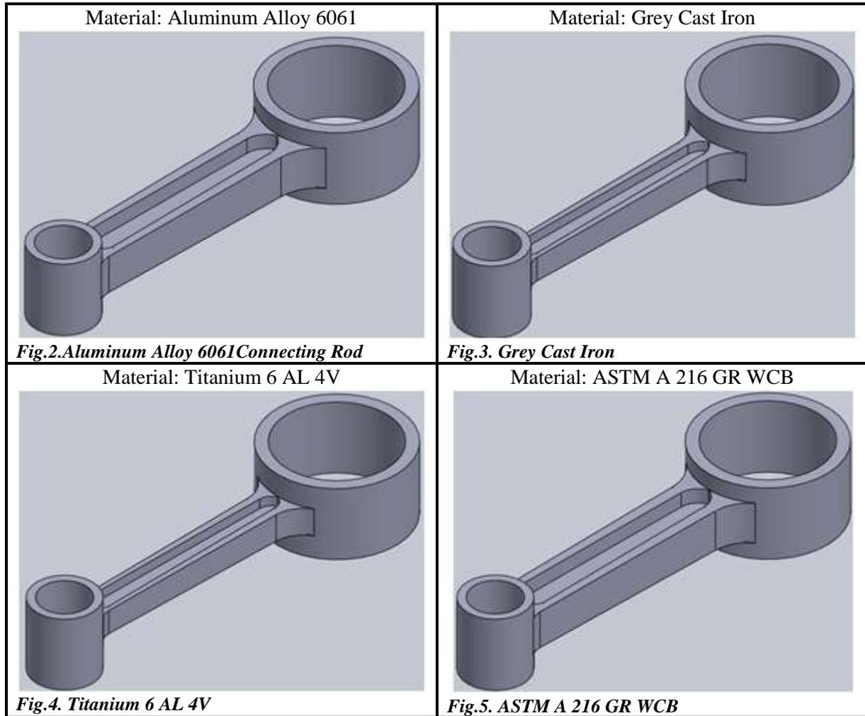
Fig.2. Aluminum Alloy 6061 Connecting Rod
