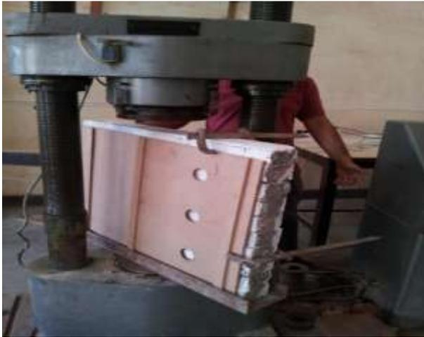
**Figure 11.** Carrying wall on testing machine by wood panels
