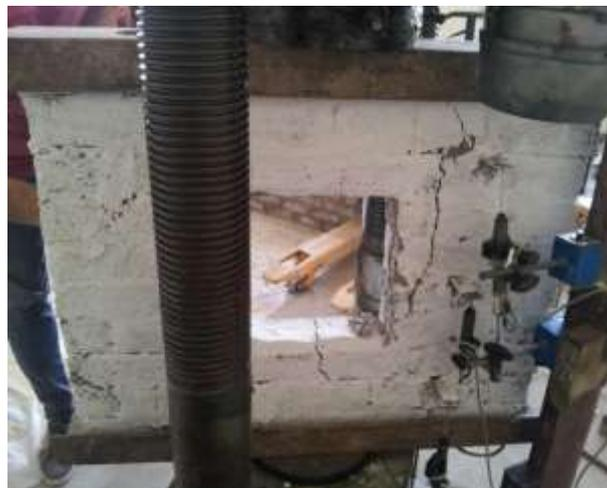
**Figure 2.** Cracks around window opening
