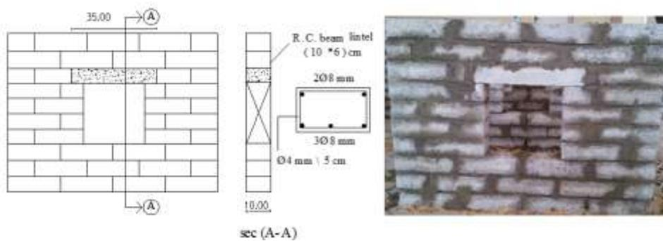
**Figure 4.** Brick wall with R.C. lintel 35 cm (control wall)
