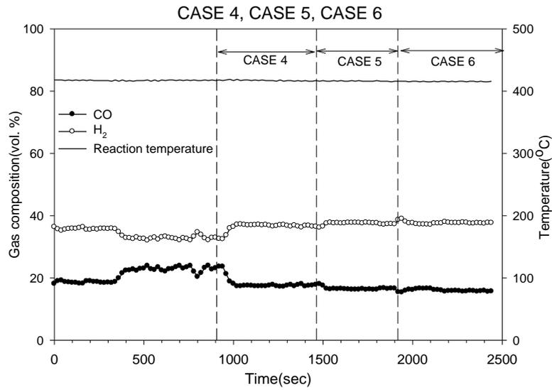
Fig. 7. Gas composition after reaction of CASE 4~CASE 6
