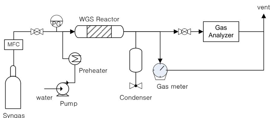
Fig. 2. Schematic diagram of lab-scale WGS reactor
