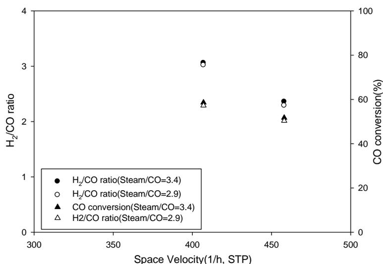
Fig. 10. Influence of space velocity on H<sub>2</sub>/CO ratio and CO conversion
