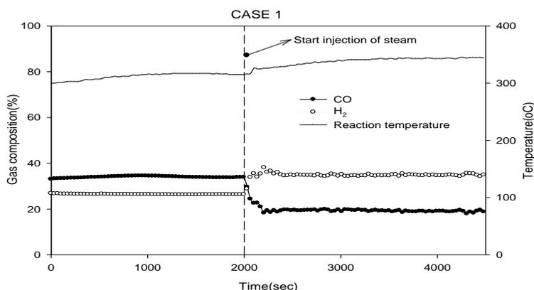
Fig. 5. Gas composition after reaction of CASE 1
