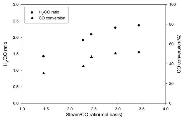
Fig. 10. Influence of steam/CO ratio on H<sub>2</sub>/CO ratio and CO conversion
