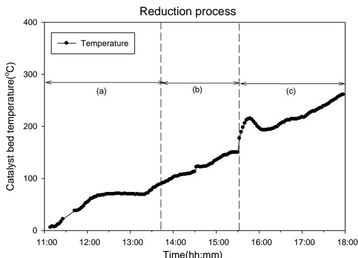
Fig. 4. Temperature profile during reduction process
