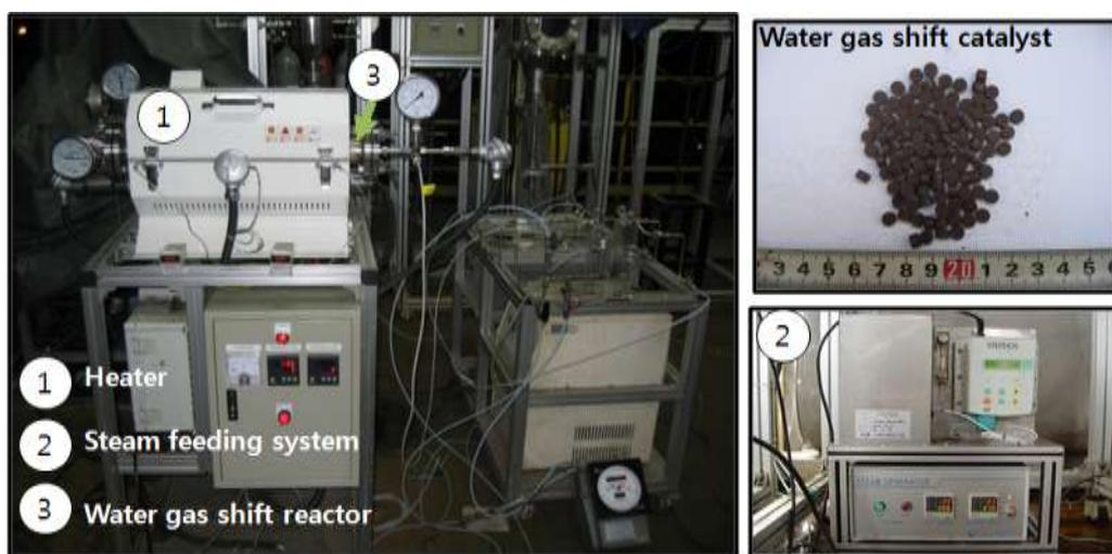
Fig. 3. Picture of lab-scale WGS reactor
