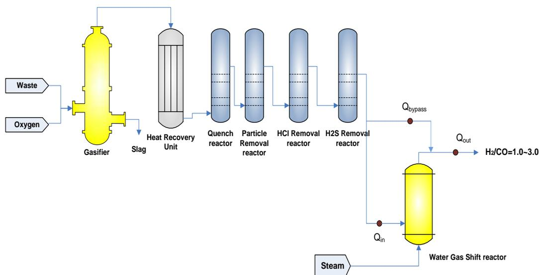
**Fig. 1.** Waste gasification system including WGS unit
