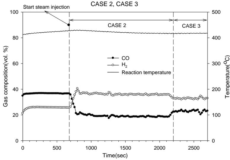
Fig. 6. Gas composition after reaction of CASE 2 and CASE 3
