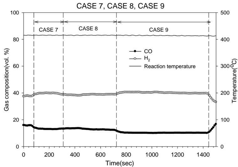
Fig. 8. Gas composition after reaction of CASE 7~CASE 9
