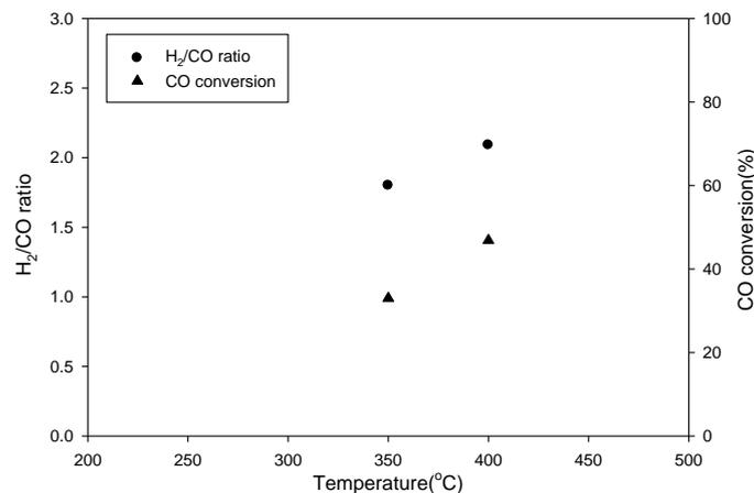
Fig. 9. Influence of temperature on H<sub>2</sub>/CO ratio and CO conversion
