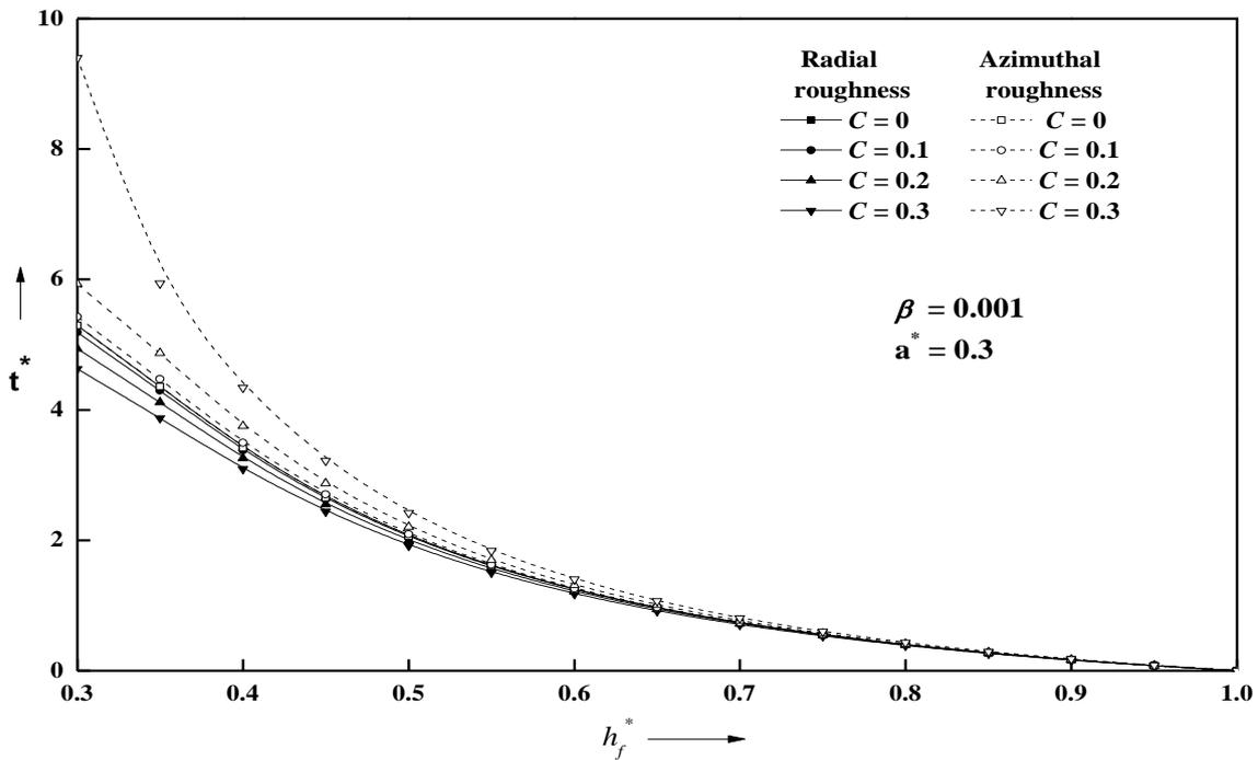
Figure 7. Variation of squeeze film time  $t^*$  with film thickness  $h_f^*$  for different values of  $C$  with  $a^* = 0.3$  and  $\beta = 0.001$
