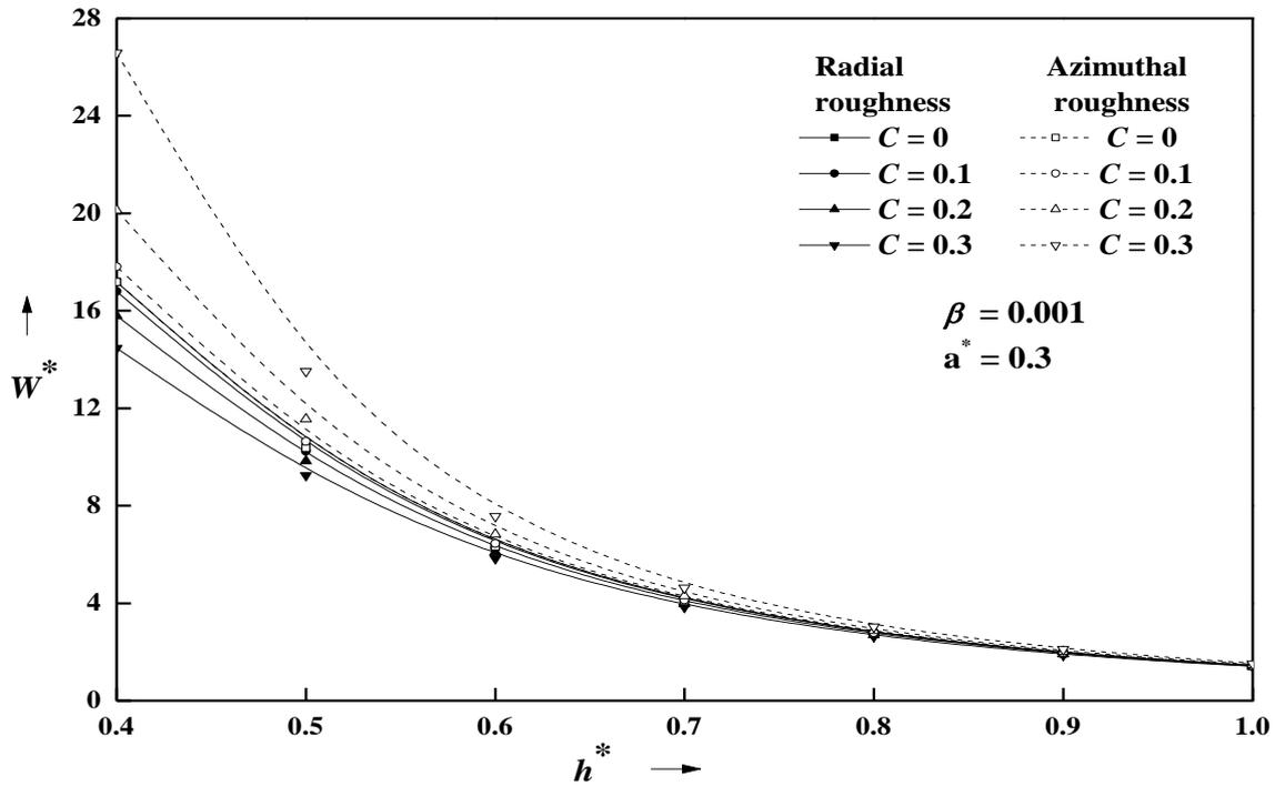
Figure 5. Variation of non-dimensional load carrying capacity  $w^*$  with  $h^*$  for different values of  $C$  with  $a^* = 0.3$  and  $\beta = 0.001$ .
