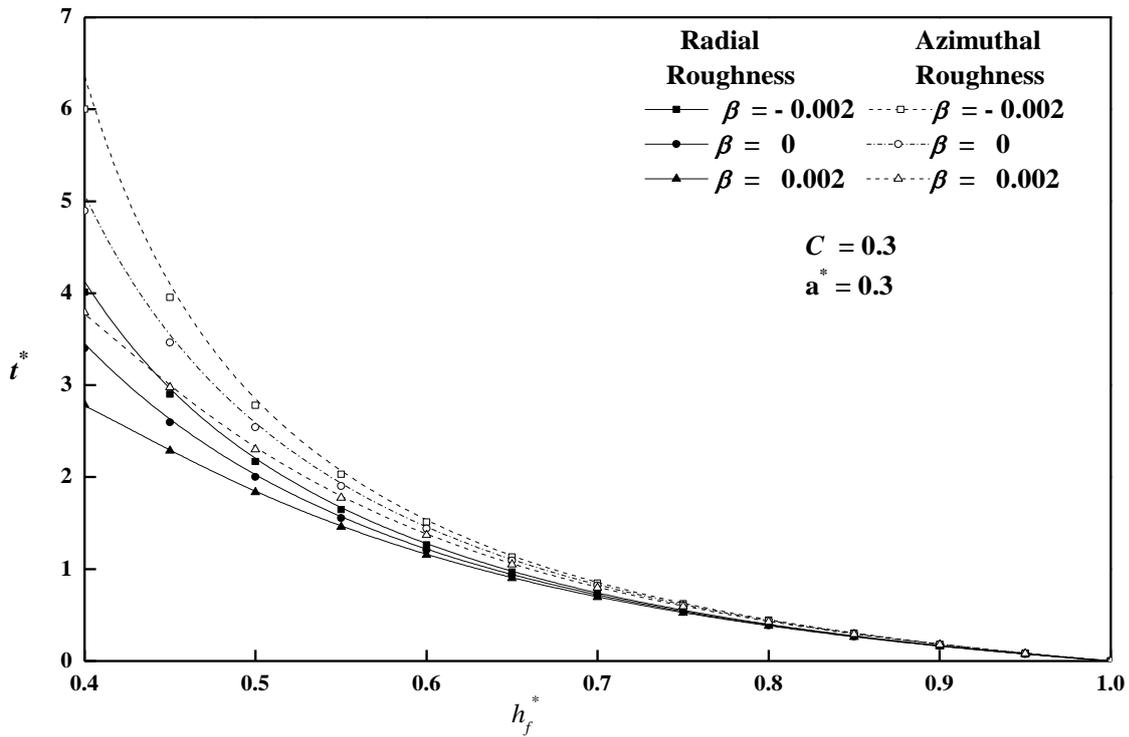
Figure 6. Variation of squeeze film time  $t^*$  with film thickness  $h^*$  for different values of  $\beta$  with  $a^* = 0.3$  and  $C = 0.3$
