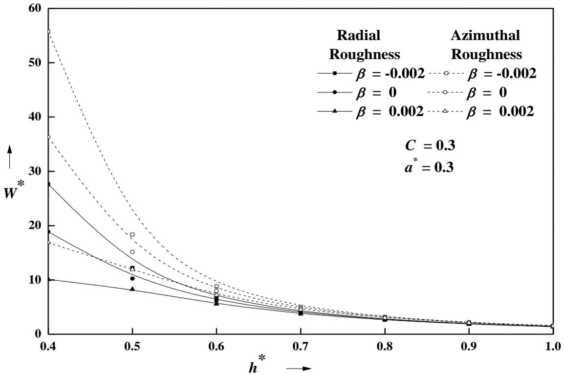
Figure 4. Variation of non-dimensional load carrying capacity  $w^*$  with film thickness  $h^*$  for different values of  $\beta$  with  $a^* = 0.3$  and  $C = 0.3$
