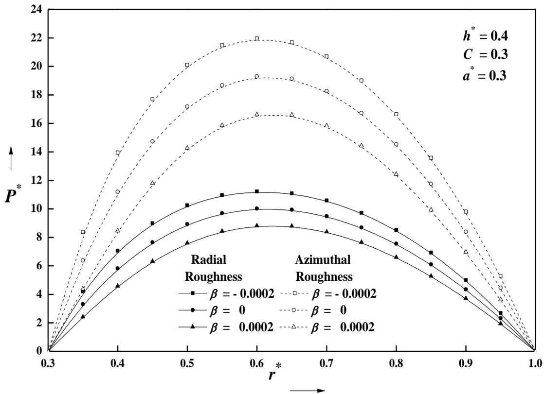
Figure 2. Variation of non-dimensional pressure  $P^*$  with  $r^*$  for different values of  $\beta$  with  $h^* = 0.4, a^* = 0.3$  and  $C = 0.3$
