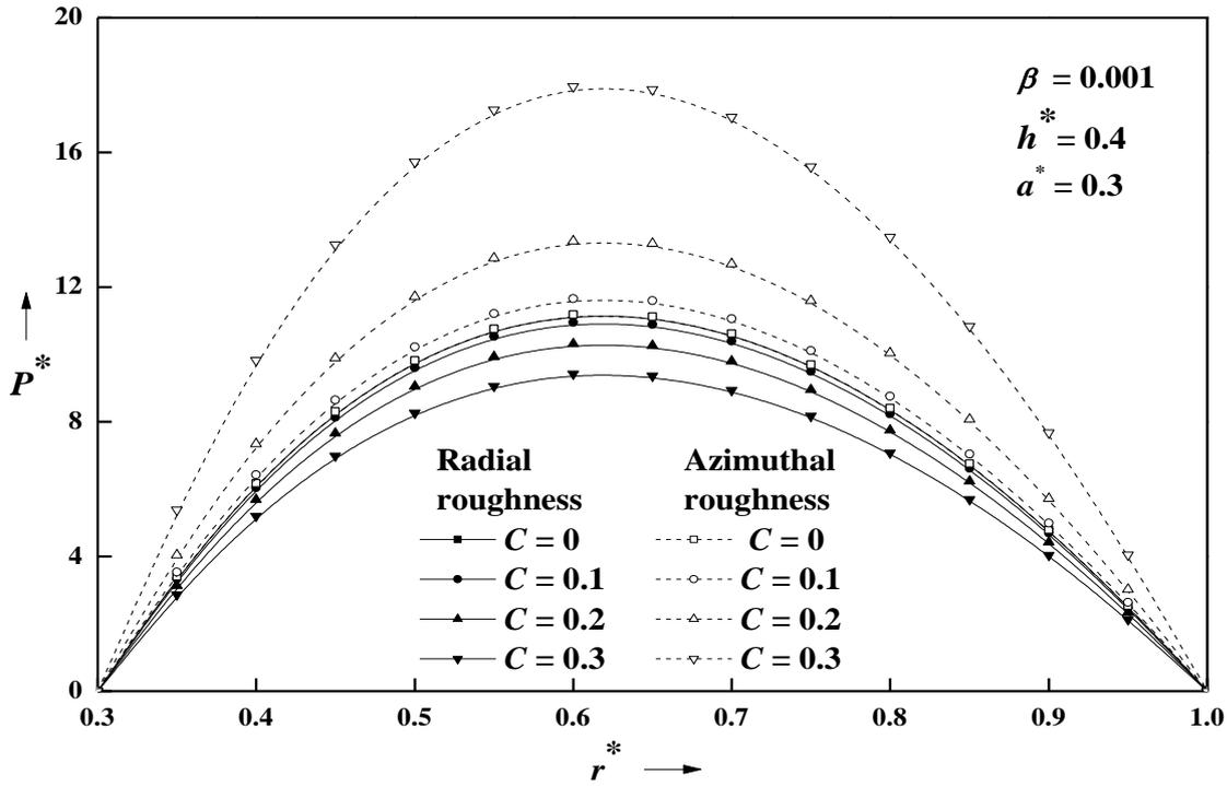
Figure 3. Variation of non-dimensional pressure  $P^*$  with  $r^*$  for different values of  $C$  with  $\beta = 0.001$ ,  $a^* = 0.3$  and  $h^* = 0.4$
