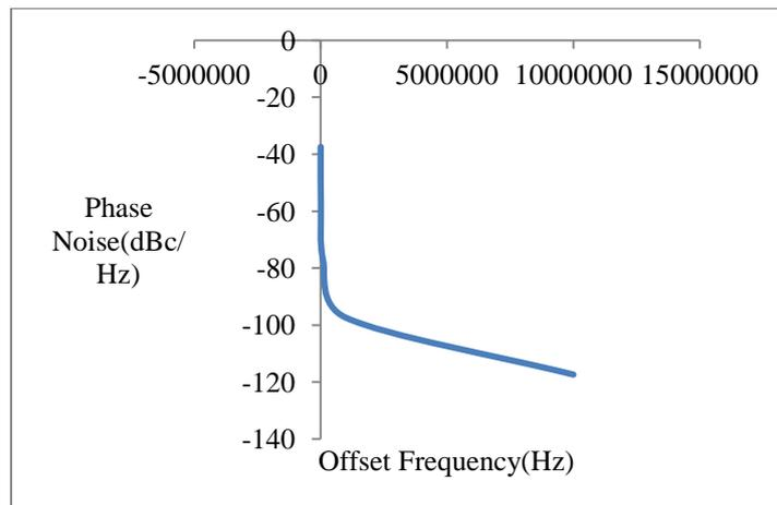
**Fig.5** Phase noise vs. Offset frequency graph
