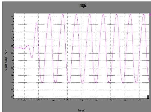
**Fig.7(a)** Oscillation at  $V_{tune} = 0V$
