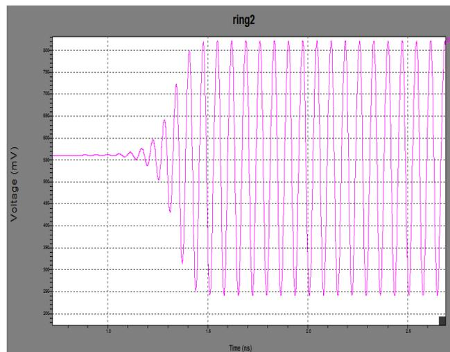
**Fig.7 (b)** Oscillation at  $V_{tune}=3.4V$
