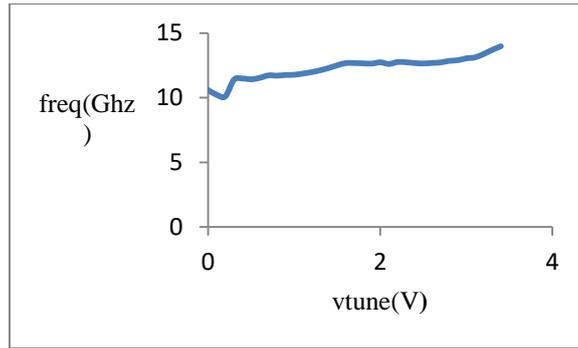
**Fig.6.** Tuning voltage vs. Frequency graph
