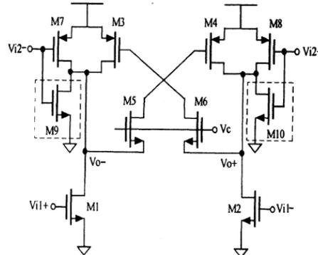
Fig.1 Delay cell with pre-charge MOSFET[2]
