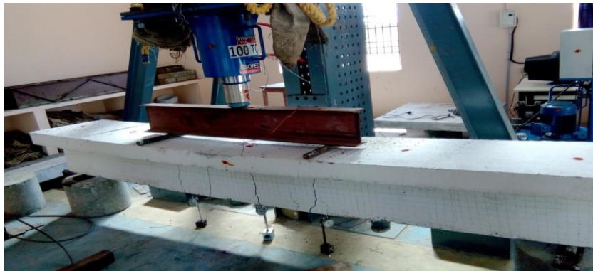
Fig 8: Flexural Tested on Tee Beam
