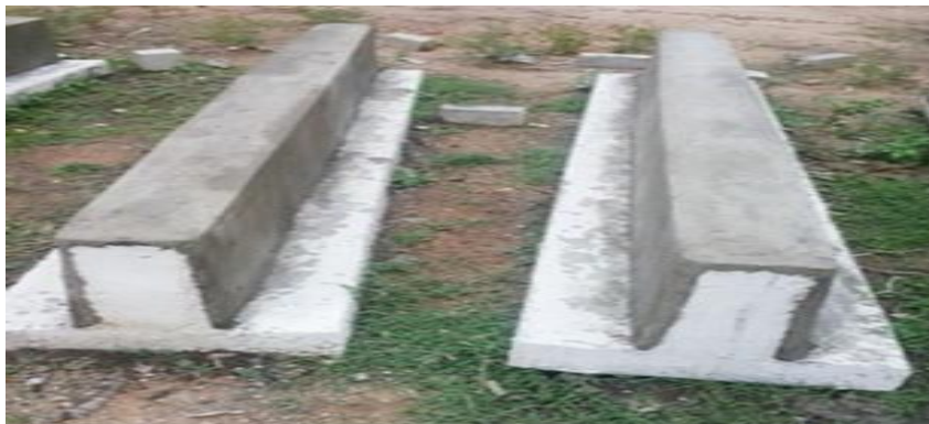
Fig 9: Pre – loaded Beams are retrofitting all faces of web T Beams ( B_{RW} )
