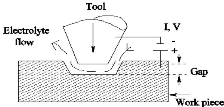
Fig. 1. Schematic diagram showing the operation of ECM
