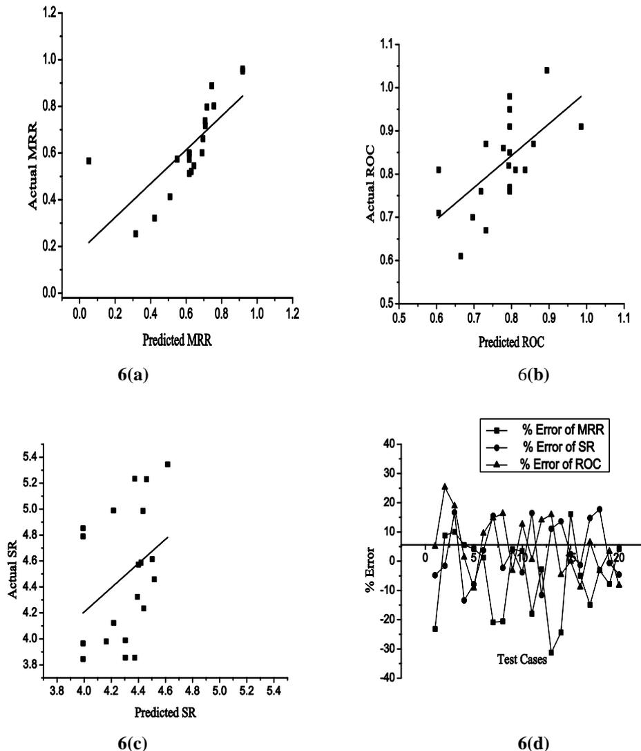
**Fig. 6.** Test cases experimental results for FLA-1: (a) actual MRR vs model predicted MRR (b) actual ROC vs model predicted ROC (c) actual SR vs model predicted SR (d) percentage deviation in prediction of all the responses.
