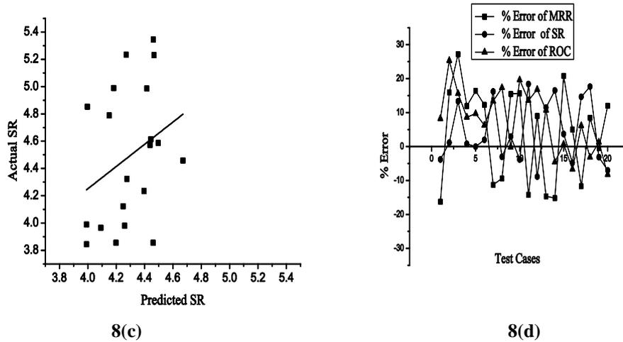
**Fig. 8.** Test cases experimental results for FLA-2: (a) actual MRR vs model predicted MRR (b) actual ROC vs model predicted ROC (c) actual SR vs model predicted SR (d) percentage deviation in prediction of all the responses.
