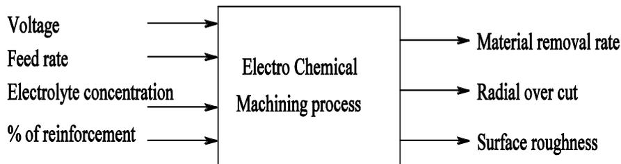
Fig. 2. Input and output parameters of electrochemical machining process
