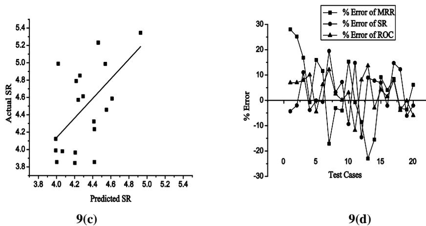
**Fig. 9.** Test cases experimental results for FLA-3: (a)actual MRR vs model predicted MRR (b)actual ROC vs model predicted ROC (c)actual SR vs model predicted SR (d)percentage deviation in prediction of all the responses.
