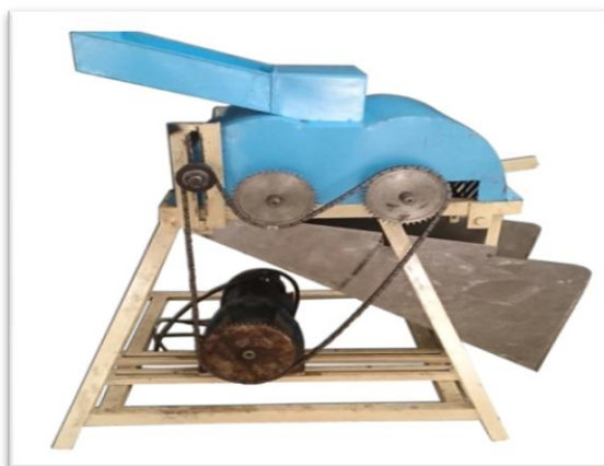
Fig: 5 Palmyrah palm jaggery disintegrating unit
