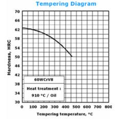
Figure 2. 2550 Tempering Diagram of Cold Work Toll Steel [9].
