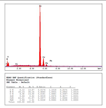
Figure 13. General EDS Analysis taken from lateral surface of CrN coated specimen
