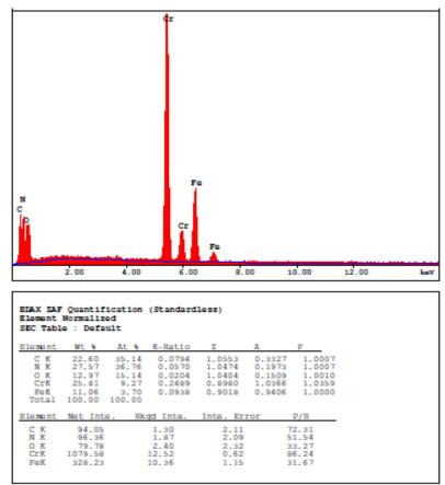
Figure 12. EDS Analysis taken from coating surface in section of CrN coated specimen
