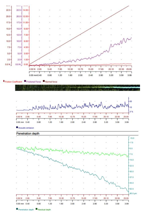
Figure 14. Scratch Test Results applied to TiN Coated specimens (friction graph, microscopic image of scratch, and acoustic emission graph)
