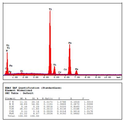
Figure 10. EDS Analysis taken from coating surface in section of TiN coated specimen
