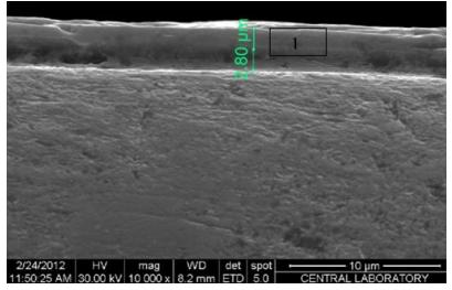
Figure 9. SEM image taken from section of TiN Coated specimen
