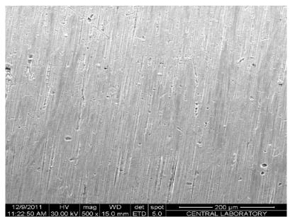
Figure 8. SEM image taken from lateral surface of CrN Coated specimen
