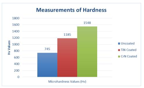
Figure 3. Microhardness values of specimens
