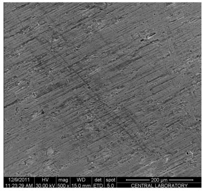
Figure 6. SEM image taken from lateral surface of TiN Coated specimen
