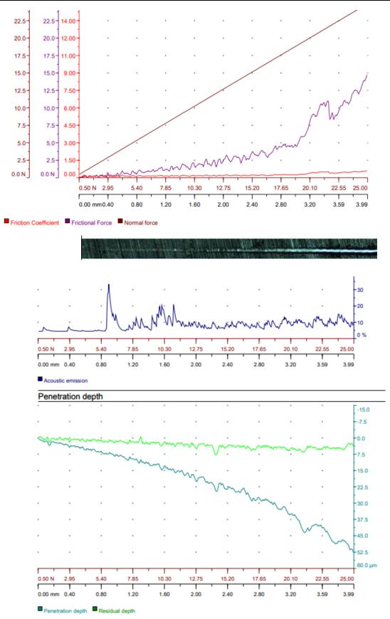
Figure 15. Scratch Test Results applied to CrN Coated specimens (friction graph, microscopic image of scratch, and acoustic emission graph)
