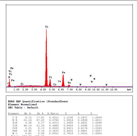
Figure 7. General EDS Analysis taken from lateral surface of TiN coated specimen
