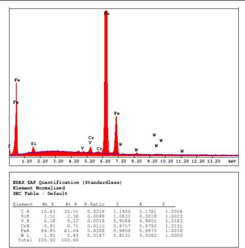
Figure 5. General EDS Analysis taken from lateral surface of non-coated specimen
