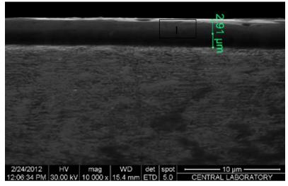
Figure 11. SEM image taken from section of CrN Coated specimen
