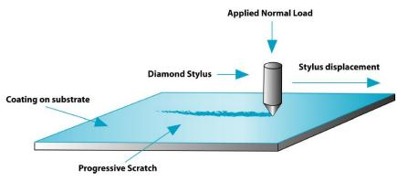
Figure 1. Schematic Test Method [7].
