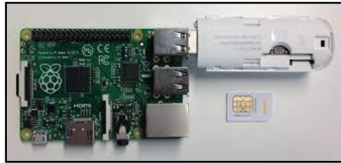
Fig. 11. Raspberry PI Interface with USB GSM module
