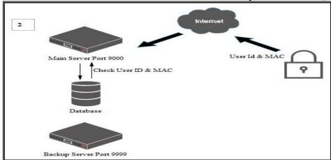
Figure 2 - First Lock Is Connecting To Main Server.
