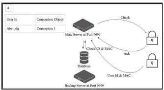
All The Process Repeats Whenever A New Lock Device Becomes Online (Figure-4). Server Always Keeps The **Figure 4 -** Second Lock Is Connecting To Main Server.
