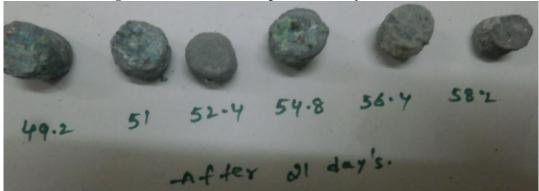
Fig4.4B.Corrosion Test Samples After 21 Days
