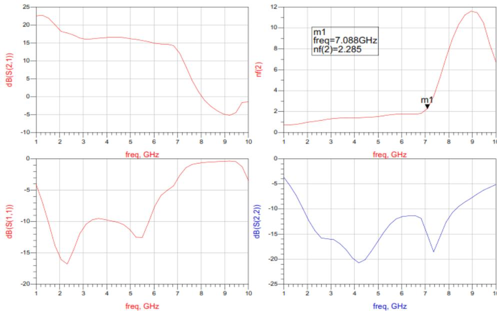
Figure 7. Collective Results Of The Active Load Topology LNA
