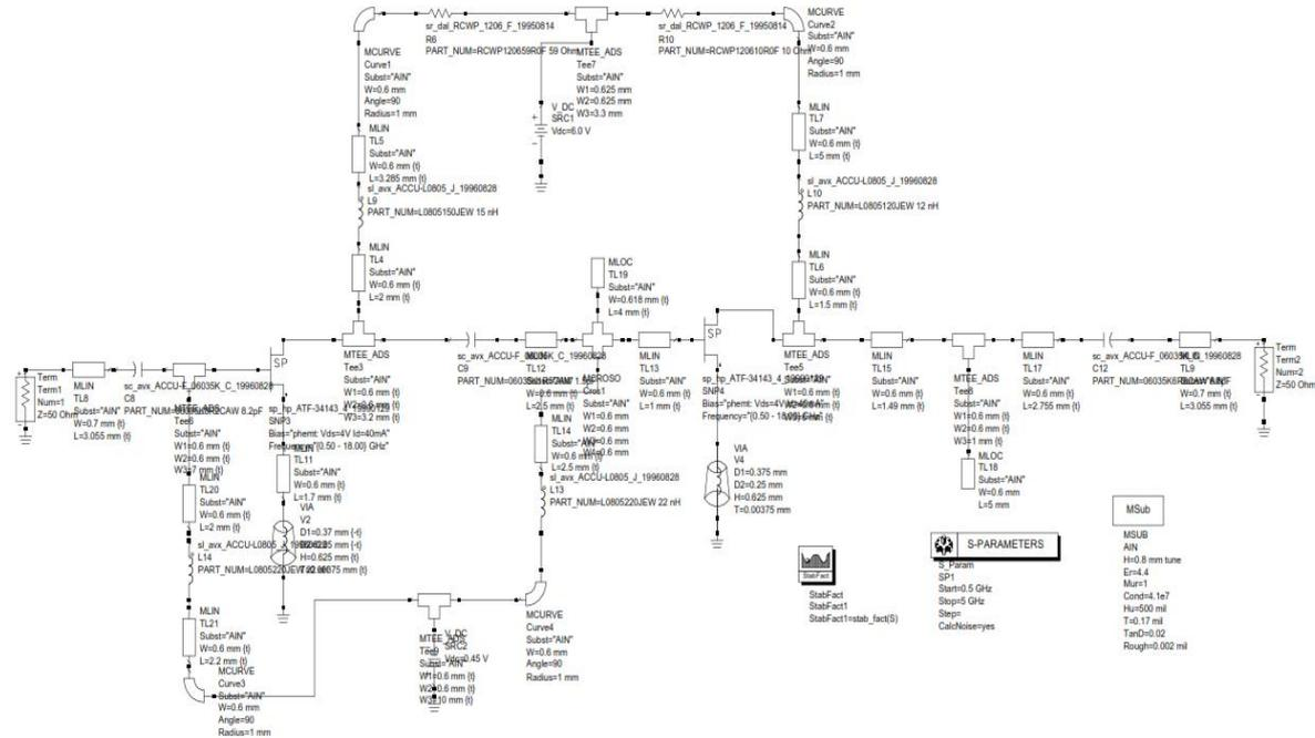
Figure 4. Circuit Schematic Of Cascaded Series Capacitor And Source Inductance
