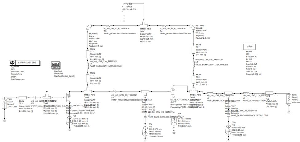
Figure 1. Shows Cascaded Amplifier Using ATF 34143 With LC Matching Network
