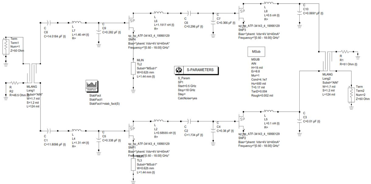
Figure 8. Schematic Of LNA Design Using Balanced Amplifier Technique
