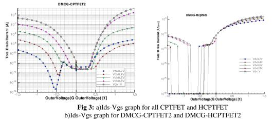
**Fig 4.** a) Comparative plots of transfer characteristics of DMCG-CPTFET2 b) Comparative plots of transfer characteristics of DMCG-HCPTFET2
