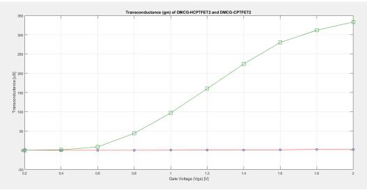
Fig 5: Plot for transconductance of DMCG-CPTFET2 and DMCG-HCPTFET2
