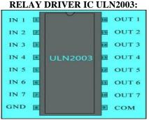
Fig. Pin Diagram Of Relay Driver
