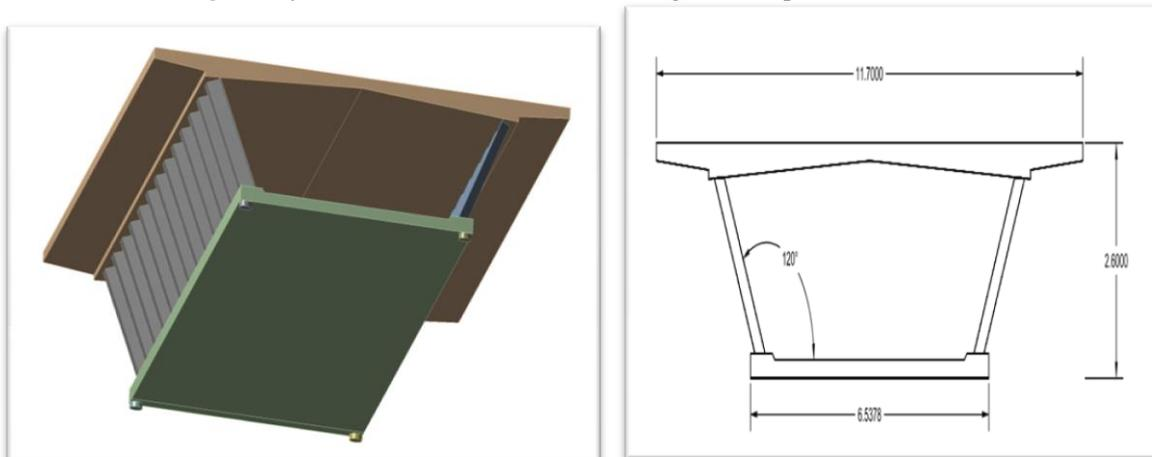
Fig.2 Ansys And Autocadd Model Of Trapezoidal Composite Box Girder
