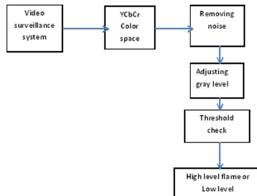
Fig.1. Flow Chart Of Proposed Algorithm For Fire Detection
