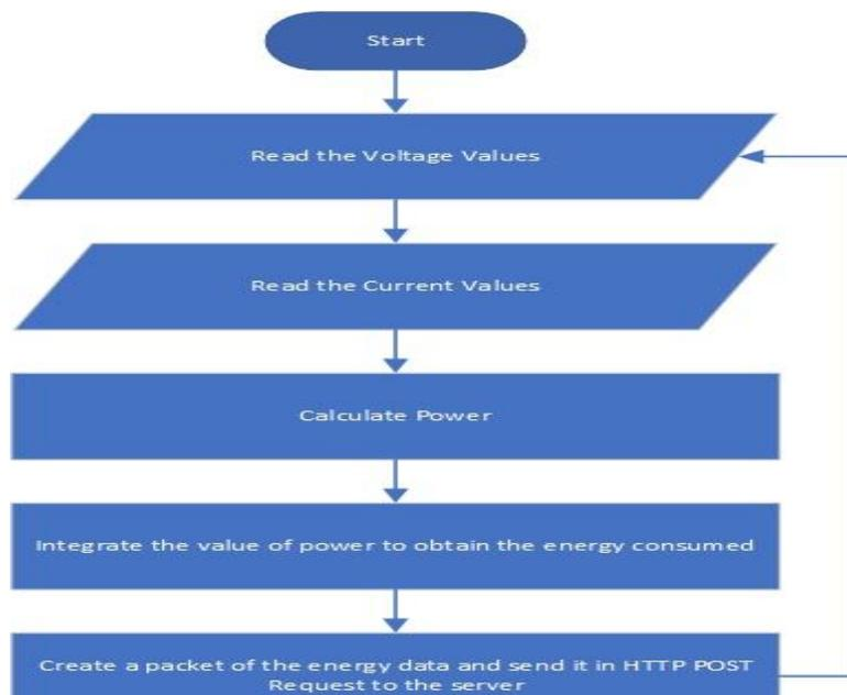
**Figure 2: Flow Chart Explaining The Logic Of The Firmware**
