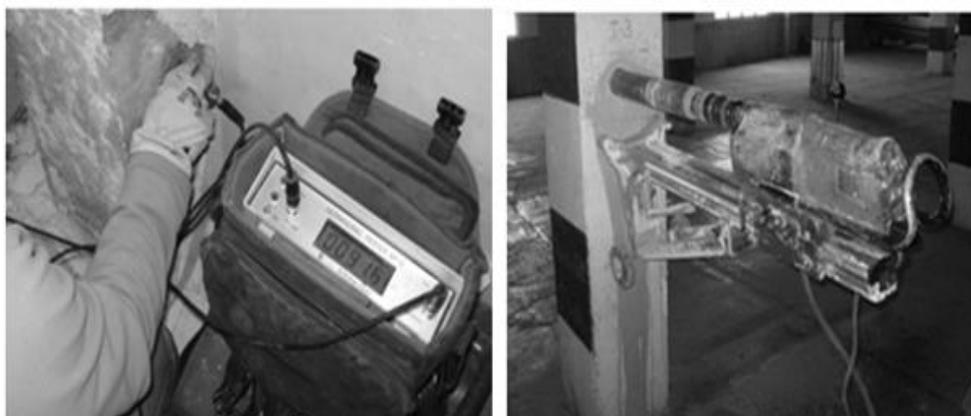
**Figure 1** Ultrasonic Testing Process (Left). Moment Of Extraction Of A Test Specimen (Right)
