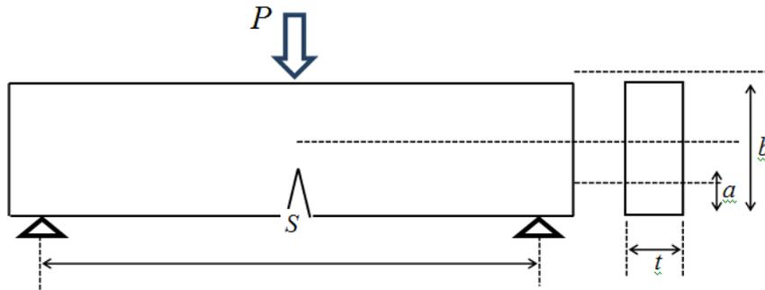
Fig.2 Three point bending test
