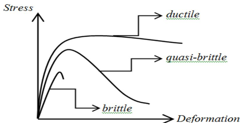
Fig 1. Transition of brittle to ductile failure
