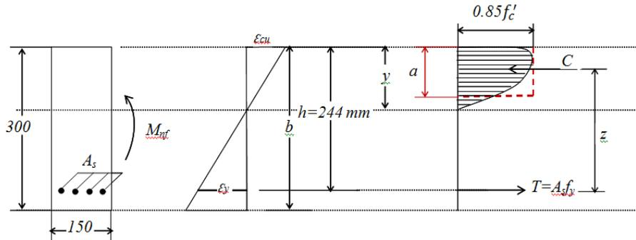
Fig.5 Beam with balancing reinforcement
