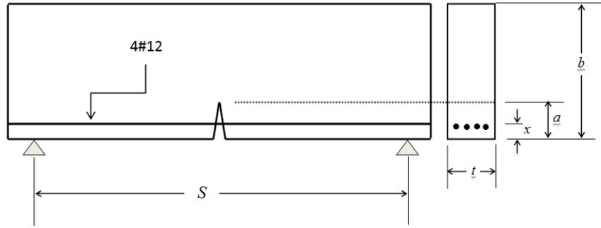
Fig. 4 Three point bending beam with tensile opening
