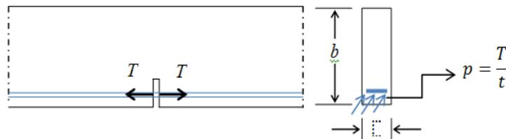
**Fig.3 Wedge forces of a single crack reinforced beam**
