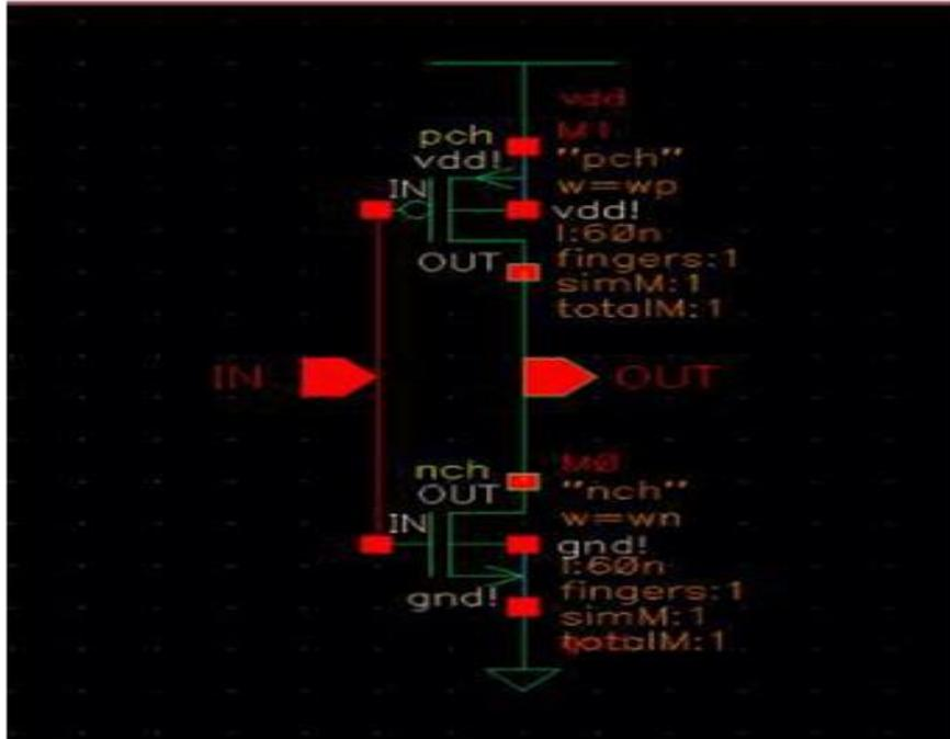
**Fig:3** Schematic diagram of CMOS inverter
