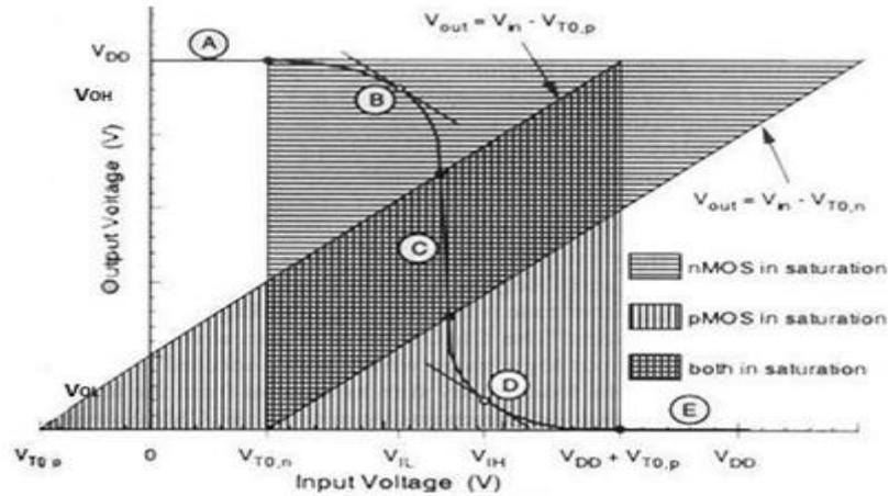
Fig 2: Operating region of n-MOS and p-MOS transistor [1]
