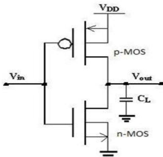
Fig 1: Structure of CMOS inverter
