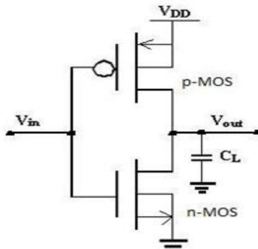
Fig 1: Structure of CMOS inverter
