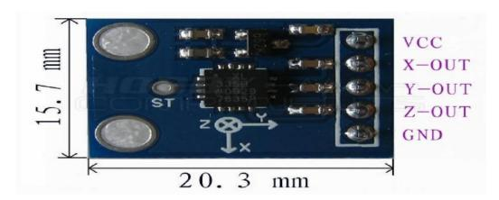
GY-61 DXL335 3-Axis Accelerometer Module is a three axis accelerometer sensor module based on ADXL335 integrated circuit. It is a triple axis accelerometer with low noise and power consumption. The sensor has a full sensing range of  $\pm$  3g. It can measure the static acceleration of gravity in tilt-sensing applications, as well as dynamic acceleration resulting from motion, shock, or vibration.
