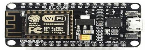
TheNodeMCU (Node Microcontroller Unit) is open source software and hardware development atmosphere that is engineered around a System-on-a-Chip (SoC) referred to as the ESP8266. The ESP8266, designed and created by Espressif Systems, contains all crucial components of a computer: electronic equipment, RAM, networking (wifi), and even a modern operating system and SDK.
