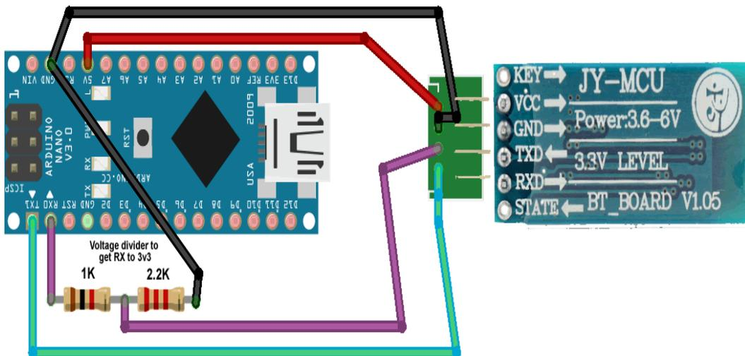
FIG. ARDUINO TO BLUETOOTH
