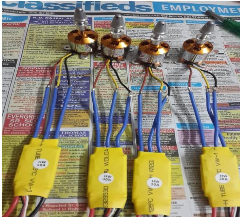
FIG. BRUSHLESS MOTOR AND ESC
