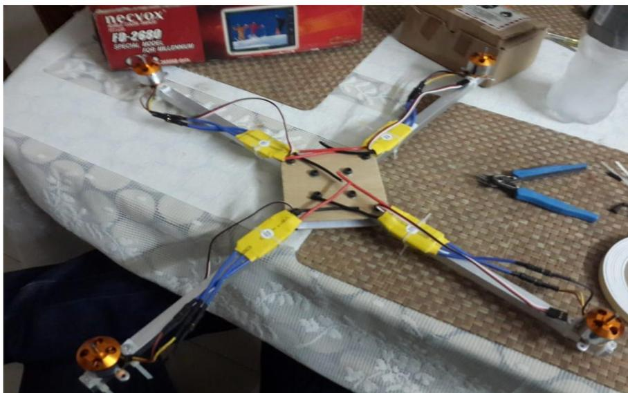
FIG. ESC CONNECT WITH EACH OTHER
