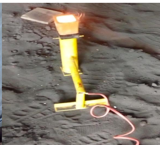
Fig 3.3 Metal poured into Cup
