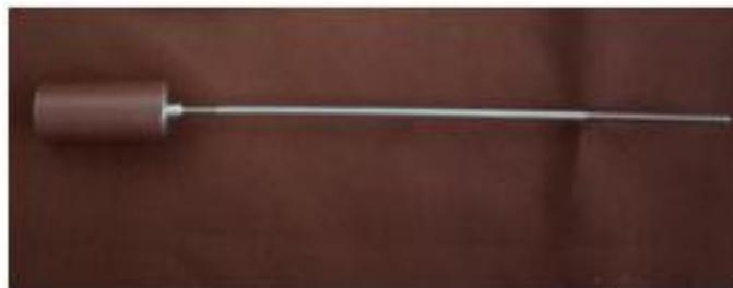
b. Piston and piston rod assembly
