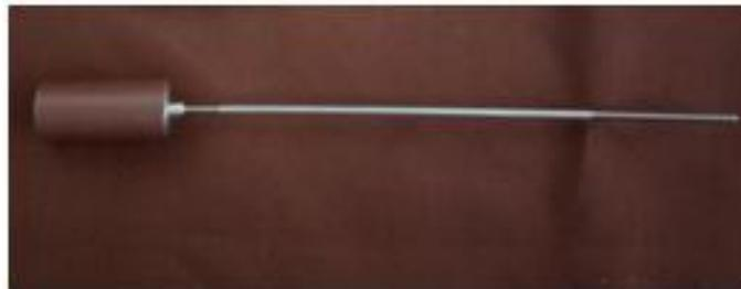
b. Piston and piston rod assembly
