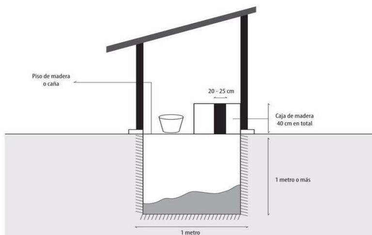
**Figure 2.** Scheme of a dry toilet.
