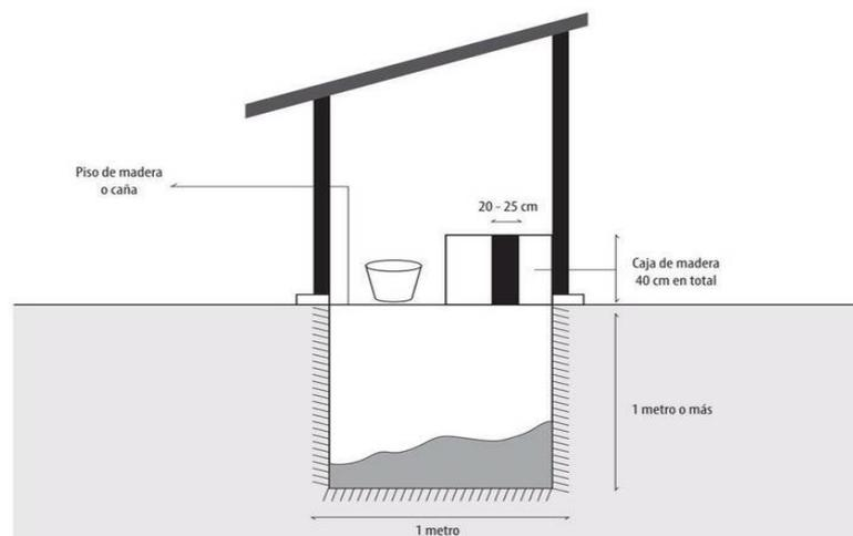
**Figure 2.** Scheme of a dry toilet.
