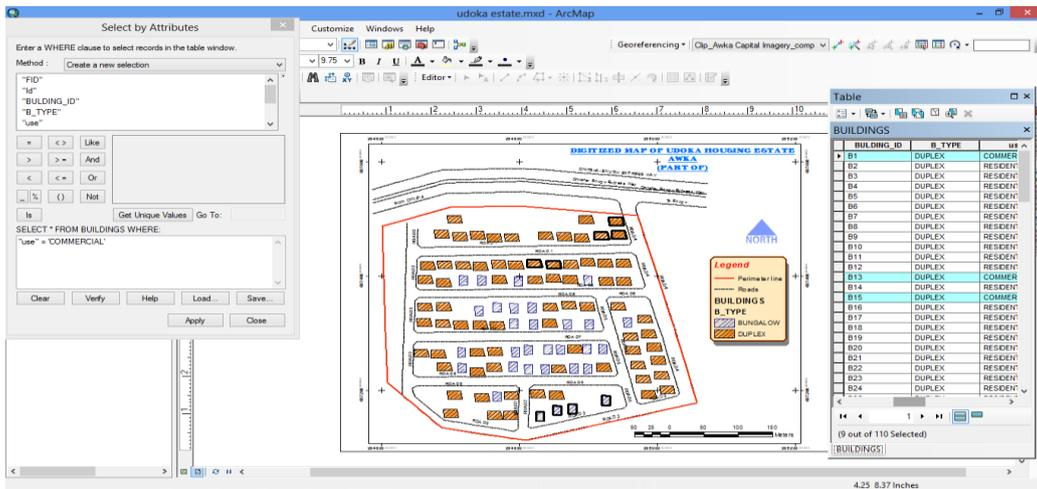
Fig. 3.3: Result of query showing building use= commercial
