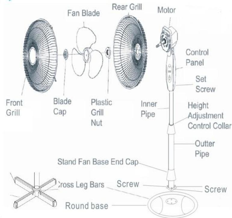
Fig. 1: Assembly of Standing Fan
