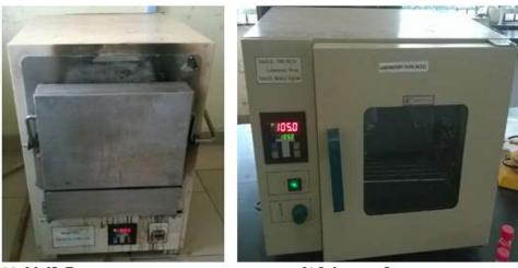
(a) Muffle Funace (b) Laboratory Oven Figure 4 Determination of Total Solid (TS) and Volatile Solid (VS)
