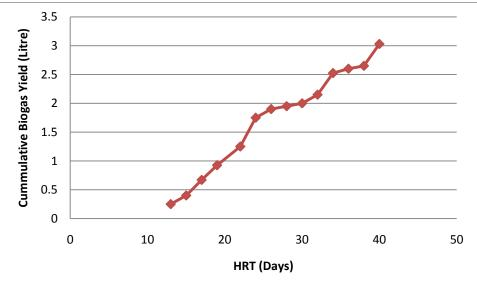
Figure 5 Plot of cumulative biogas yield against HRT
