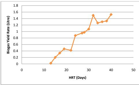
Figure 6 Plot biogas yield rate against HRT
