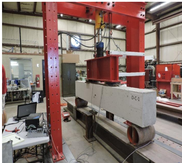
Figure 4: Beam splice test setup
