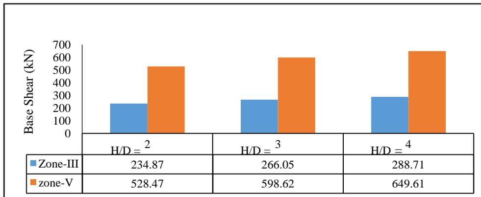
Figure. 4.1 Base Shear in Zone-III and Zone-V for various H/D ratio
