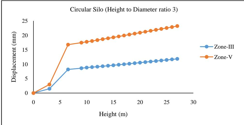
**Figure. 4.3** Maximum Lateral Displacement in X and Z Direction for Critical Load Combination for H/D ratio 3 of circular silo
