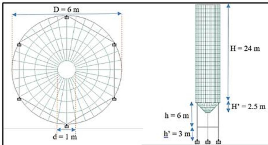
**Figure. 2.1** Top view and side view plan on circular RCC silo
