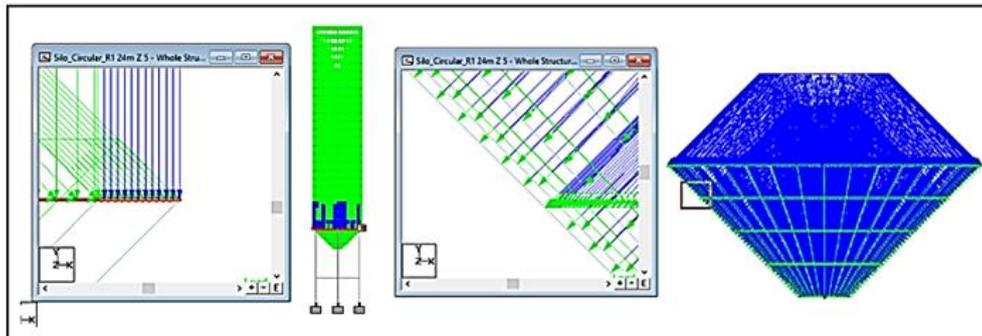
Figure 2.3 Vertical pressure on ring beam and normal pressure on hopper bottom
