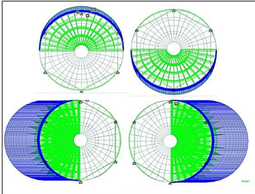
Figure 3.1 Wind pressure on silo in X and Z direction
