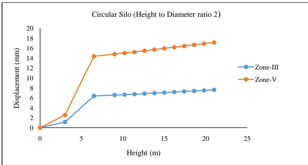
**Figure. 4.2** Maximum Lateral Displacement in X and Z Direction for Critical Load Combination for H/D ratio 2 of circular silo
