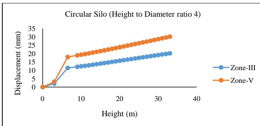
**Figure4.4** Maximum Lateral Displacement in X and Z Direction for Critical Load Combination for H/D ratio 4 of circular silo
