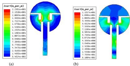
Fig. 6: Simulated surface current distributions of the proposed penta-band antenna observed at (a) 2.13 GHz, (b) 5.18 GHz
