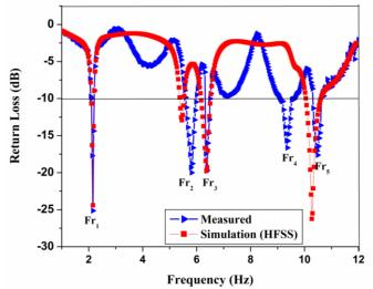
Fig. 4: Comparison of simulated and experimental return loss characteristics of modified circular patch antenna
