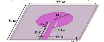
Fig. 1 Geometry of the conventional inset-fed circular microstrip antenna
