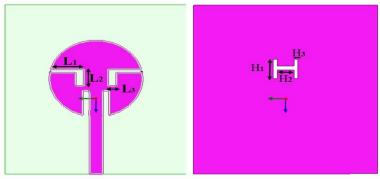
Fig. 2. Geometry of the proposed penta-band antenna
