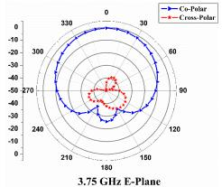
Fig. 7 Typical E-plane co and cross- polarization radiation patterns of the conventional circular microstrip patch antenna measured at 3.75 GHz
