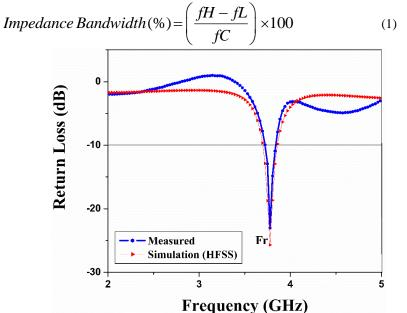
Fig. 3: Comparison of simulated and measured return loss characteristics of conventional circular patch antenna
