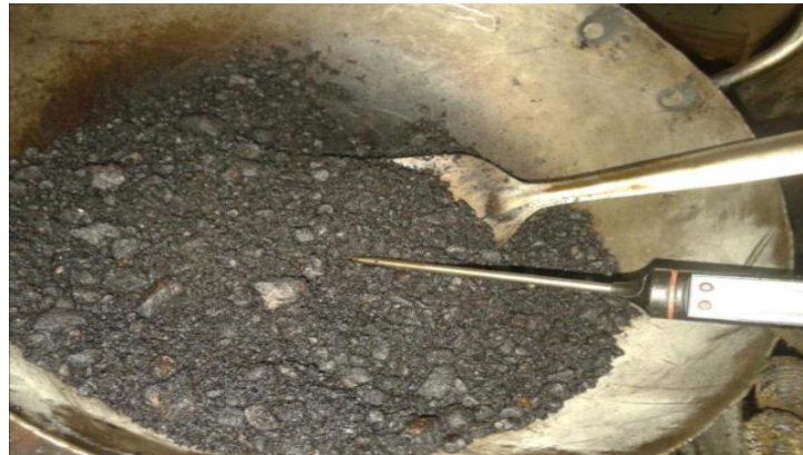
Fig: 2.Marshall Mix preparation
