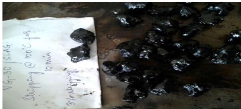
Fig: 1. Stripping test on slag aggregates
