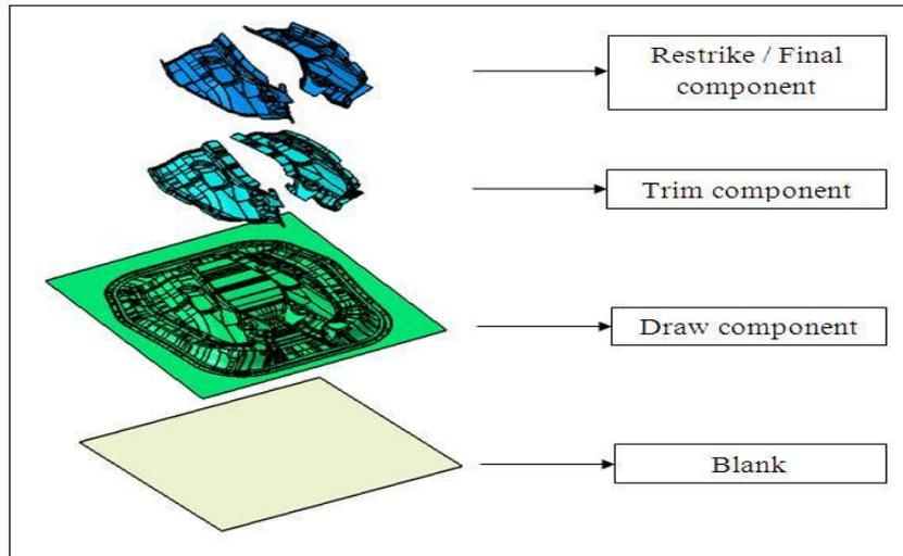
**Figure 4:** The complete process to manufacture REINF-RR END UPR-LH/RH
