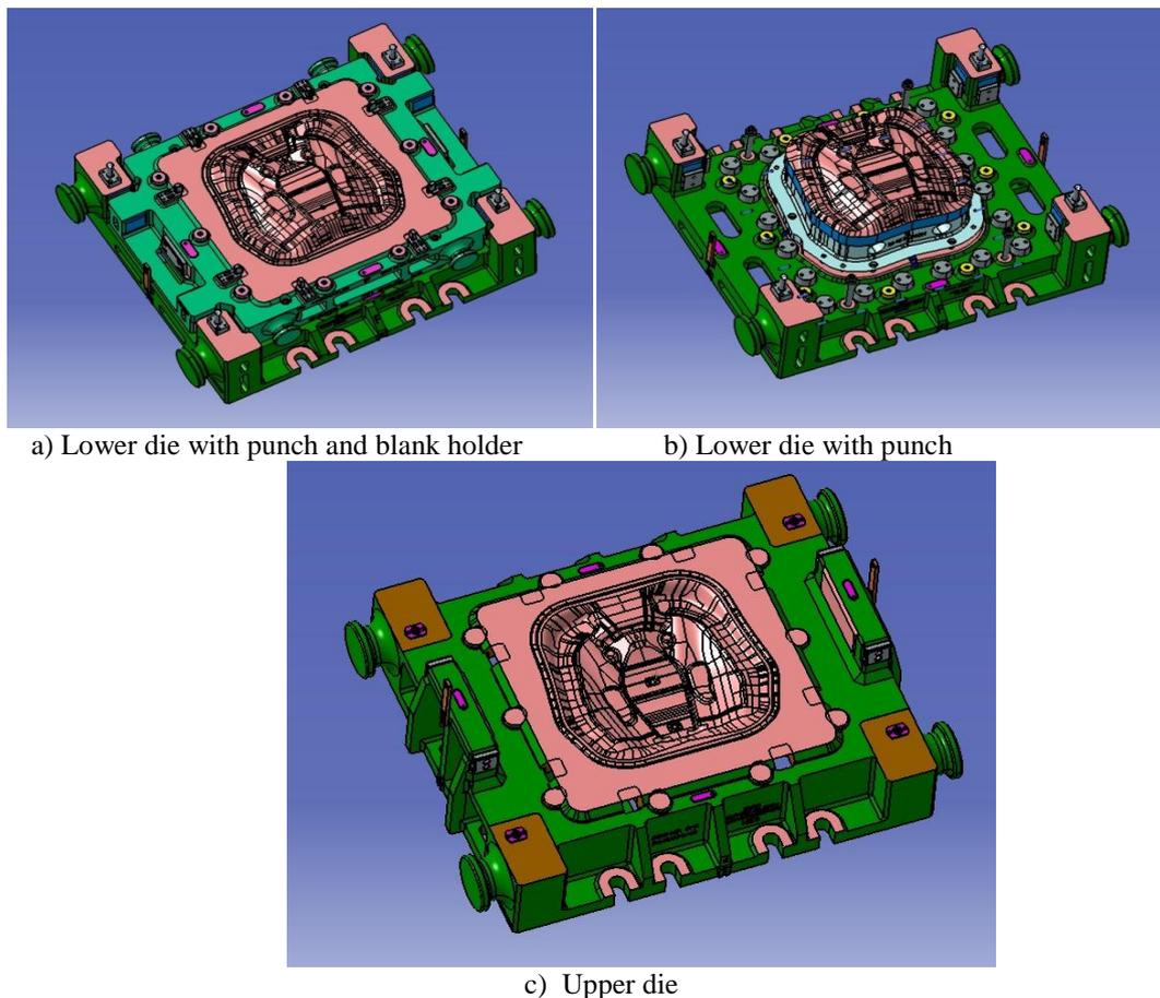
**Figure 5:** CAD model of forming tool
