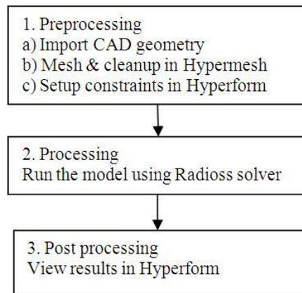
**Figure 6:** Steps in the simulation process
