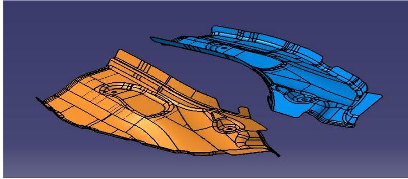
**Figure 3:** CAD model of REINF-RR END UPR-LH/RH
