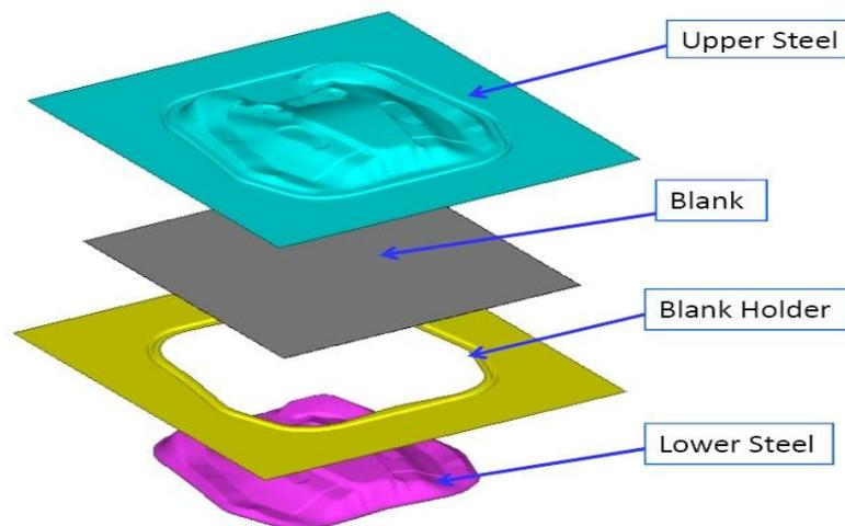
**Figure 7:** Forming tool set up
